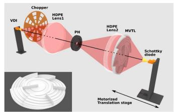
Fig. 2. Experimental setup for obtaining multiplexed THz vortex beams. The inset shows a CAD design of the MVTL experimental model.
