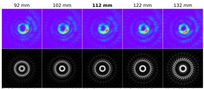
Fig. 3. Experimental results (upper row) and the numerical simulations (lower row) computed using Fresnel-Kirchhoff non-paraxial scalar diffraction theory at different transverse planes around the MVTL focal plane (z = 112 mm).
