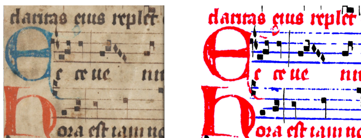
Figure 5. Example of a small portion from ground-truth data. The original image is used to extract the input feature blocks, while the labeled page indicates the categories to which each pixel belongs (white pixels mean background , black pixels mean notes , blue pixels mean staff line , and red pixels mean text ).
