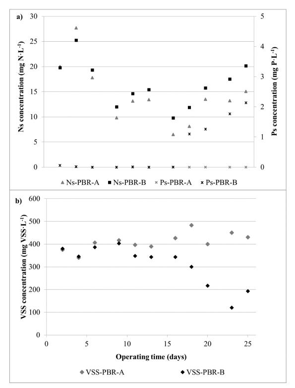
Figure 3. Evolution during Experiment 1.4 in PBR-A and PBR-B of: a) nitrogen (Ns) and phosphorus (Ps) concentrations; b) volatile suspended solids (VSS) concentration.
