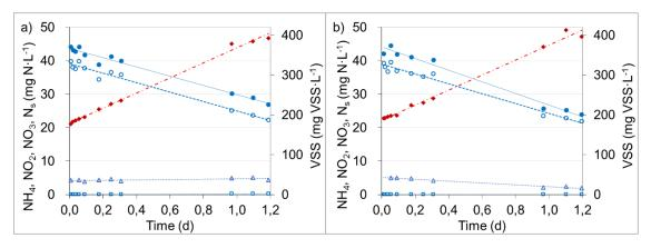
Figure A.2. Evolution of NH<sub>4</sub> ( $\circ$ ), NO<sub>2</sub> ( $\Box$ ), NO<sub>3</sub> ( $\varDelta$ ), N<sub>s</sub> ( $\bullet$ ) and VSS ( $\bullet$ ) concentration during Assay A2: a) R-A; b) R-B.
