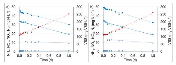
Figure A.1. Evolution of  $NH_4$  ( $\circ$ ),  $NO_2$  ( $\Box$ ),  $NO_3$  ( $\varDelta$ ),  $N_s$  ( $\bullet$ ) and VSS ( $\bullet$ ) concentration during Assay A1: a) R-A; b) R-B.
