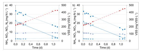
Figure A.3. Evolution of NH<sub>4</sub> ( $\circ$ ), NO<sub>2</sub> ( $\Box$ ), NO<sub>3</sub> ( $\varDelta$ ), N<sub>s</sub> ( $\bullet$ ) and VSS ( $\bullet$ ) concentration during Assay A3: a) R-A; b) R-B.
