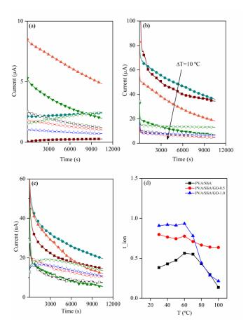
Figure 13 DC polarization current vs time plots of PVA/SSA (a), PVA/SSA/GO-0.5 (b) and PVA/SSA/GO-1.0 (c). In panel d) total ionic transference number for PVA/SSA (■), PVA/SSA/GO-0.5 (●) and PVA/SSA/GO-1.0 (▲). with temperature.
