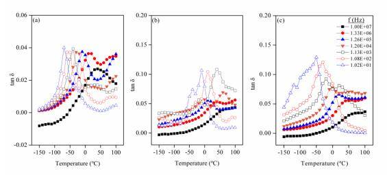
**Figure 7**. Tan  $\delta$  for a) PVA/SSA, b) PVA/SSA/GO-0.5 and c) PVA/SSA/GO-1.0 with temperature.
