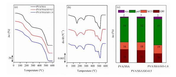
**Figure 5**. Thermogravimetric analysis and its corresponding derivative for PVA/SSA (black), PVA/SSA/GO-0.5 (red) and PVA/SSA/GO-1 (blue).
