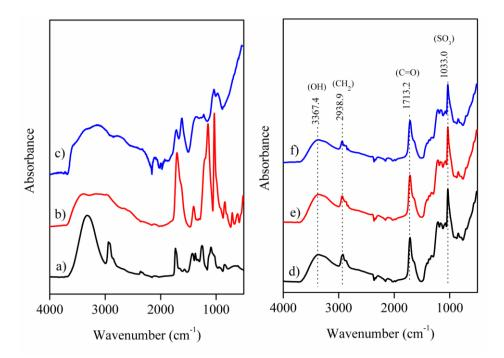
Figure 3. FT-IR spectra of a) PVA, b) SSA, c) GO, d) PVA/SSA/GO-0, e) PVA/SSA/GO-0.5 and f) PVA/SSA/GO-1.0 series polymers.
