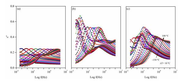
**Figure 9**. The imaginary part of dielectric permittivity for PVA/SSA (a), 0.5 wt% composite sample (b) and 1.0 wt% composite sample (c).
