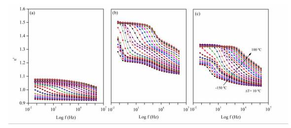
**Figure 8**. The real part of dielectric permittivity vs frequency of a) PVA/SSA, b) PVA/SSA/GO-0.5, c) PVA/SSA/GO-1.0.
