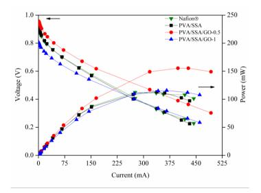
**Figure 14**. V vs I and P vs I curves for Nafion® and PVA/SSA/GO, 23 °C, pure hydrogen/oxygen, 2mg·cm<sup>-2</sup> black platinum loading, 16 cm<sup>2</sup> carbon cloth.
