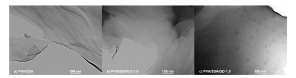
Figure 1. TEM images for (a) PVA/SSA, (b) PVA/SSA/GO-0.5, and (c) PVA/SSA/GO-1.0.
