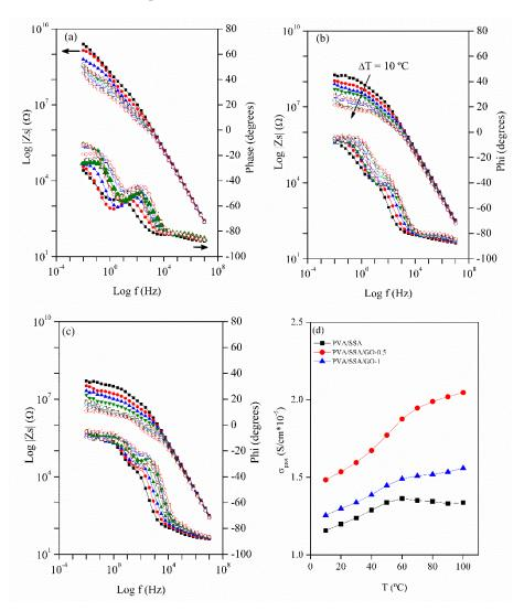
Figure 12. DC Conductivity vs f for PVA/SSA (a), 0.5 wt% composite sample (b), and 1.0 wt % composite sample (c). In panel (d) protonic conductivity evolution for PVA/SSA (■), PVA/SSA/GO-0.5 (●) and PVA/SSA/GO-1.0 (▲) with temperature.
