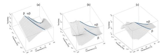
Figure 6. Frequency and temperature dependence of tan  $\delta$  for a) PVA/SSA, b) PVA/SSA/GO-0.5 and c) PVA/SSA/GO-1.0.
