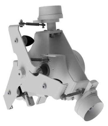
Figure 10. CAD model of the passive pitch system.
