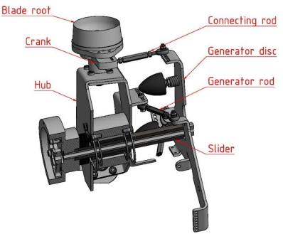
Figure 7. Main components of the passive pitch system.
