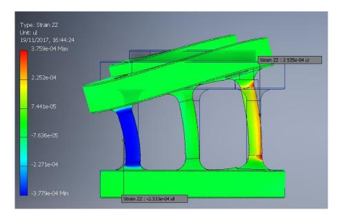
Figure 31. Strain values from the stress analysis for the bending moment sensor under pure bending moment.
