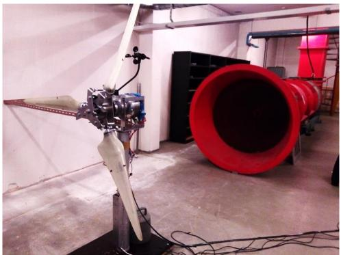
Figure 42. Wind turbine prepared for being tested in the wind tunnel outlet.
