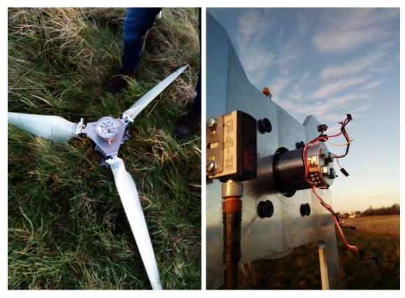
Figure 50. SWT rotor after fatigue break
