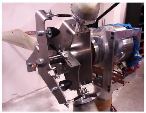
Enbreeze passive pitch system on DTU small wind turbine
