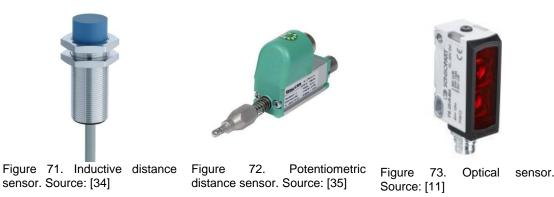
Induction sensors can measure distance ranges up to around 30mm. Unlike potentiometric and optical sensors, induction sensors need a minimum area on the surface they measure the distance. This required area, for the commercial models found, was not fulfilled, and therefore these sensors have been discarded.
