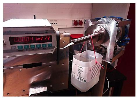
Figure 78. Crosstalk measurement. In this figure can also be seen the utilized portable amplifier SCOUT55, and the water container.
