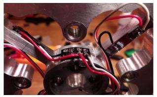
Figure 75. Intermediate phase of soldering teminals
