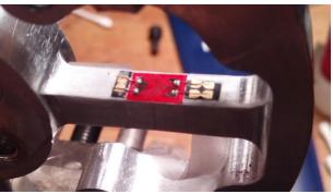
Figure 74. Shear strain gage with soldering terminals. The strain gage is slightly crooked.
