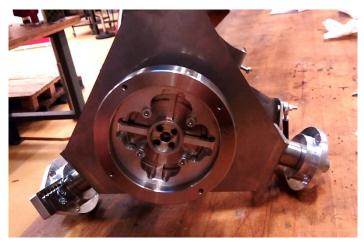
Figure 35. Thrust-torque sensor in its location in the hub.
