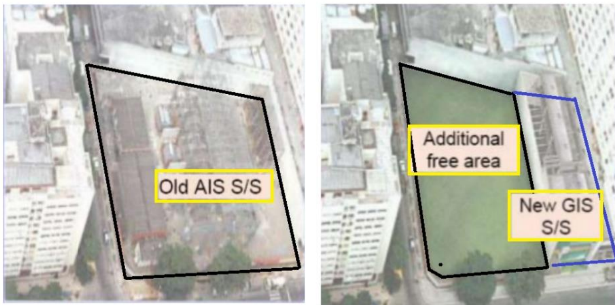
Figure 11. Real example of space use with both models, own montage with a photo of SIEMENS.
