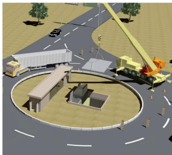
Figure 13. Substation underneath of a roundabout, by ABB.
