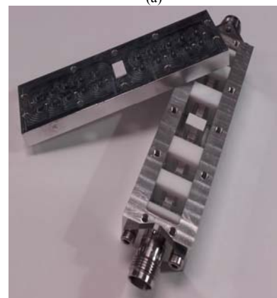
Fig. 1. Dielectric Test Device. (a) 3D-view of the stepped impedance low-pass filter. (b) Manufactured prototype.
