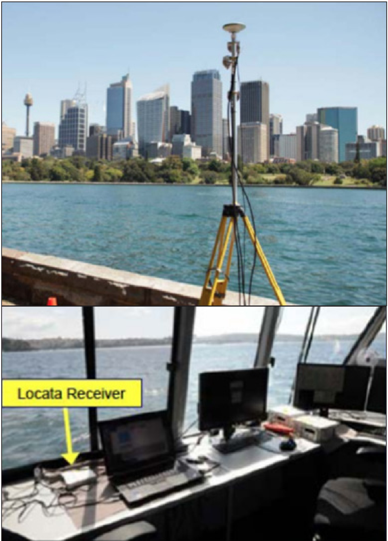
Figure 31. LocataLite situated in the Sydney harbour (up) and Locata receiver in the cabin of a ship (down)
