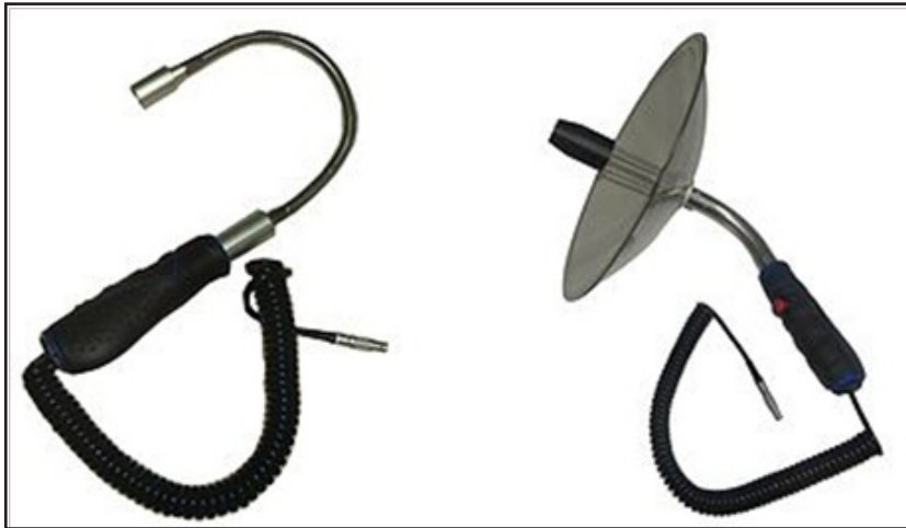
Figure 13. Handheld acoustic dish for PDetector (Partial Discharge - Power Monitoring and Diagnostic Technology, 2017)
