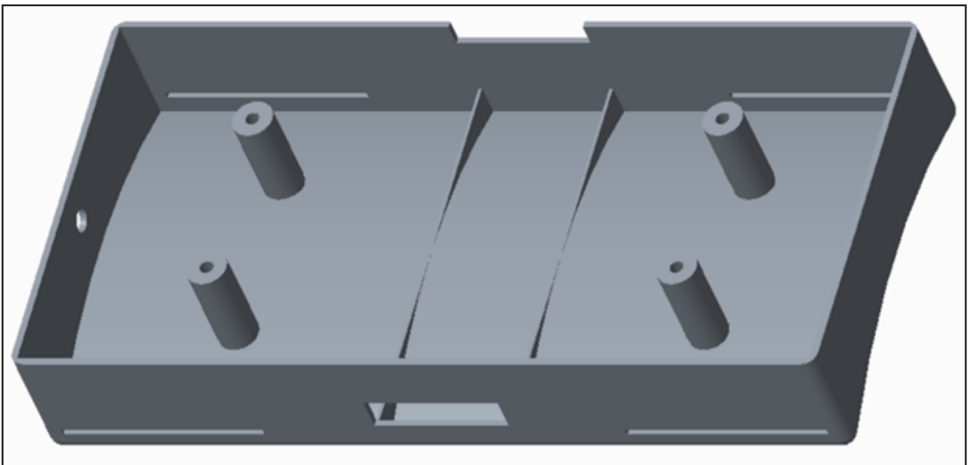
Figure 39 Bottom casing showing screw holes and clamp supports
