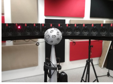
Figure 4.18. Measurement with spherical microphone
