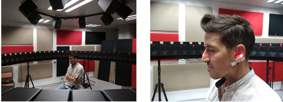
Figure 4.7. HRTF measurement process
