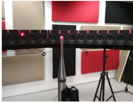
Figure 4.10. Calibration measurements with reference microphone
