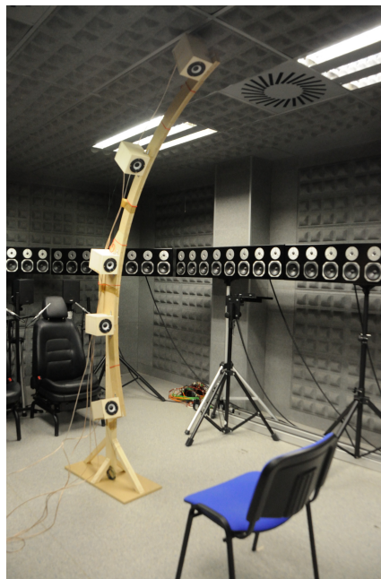
Figure 5.1. Loudspeakers for the measure of the median plane individual HRTFs
