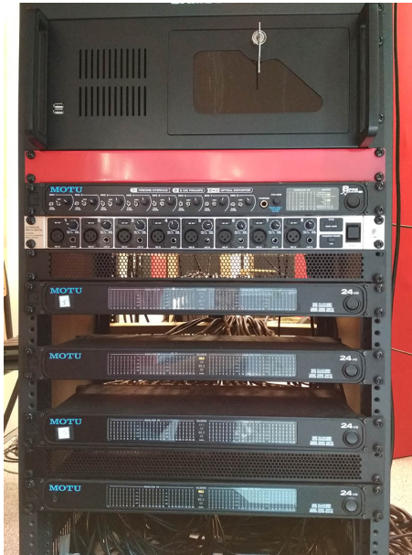
Figure 4.3. Soundcards rack used for HRTF measurements
