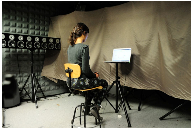
Figure 6.5. Participant seated in the listening position ready to start the test. The laptop computer with the GUI, the joystick and the acoustic curtain can be appreciated
