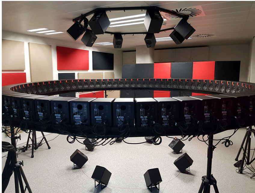
Figure 4.2. Loudspeaker set-up for HRTF measurements in the acoustically conditioned room
