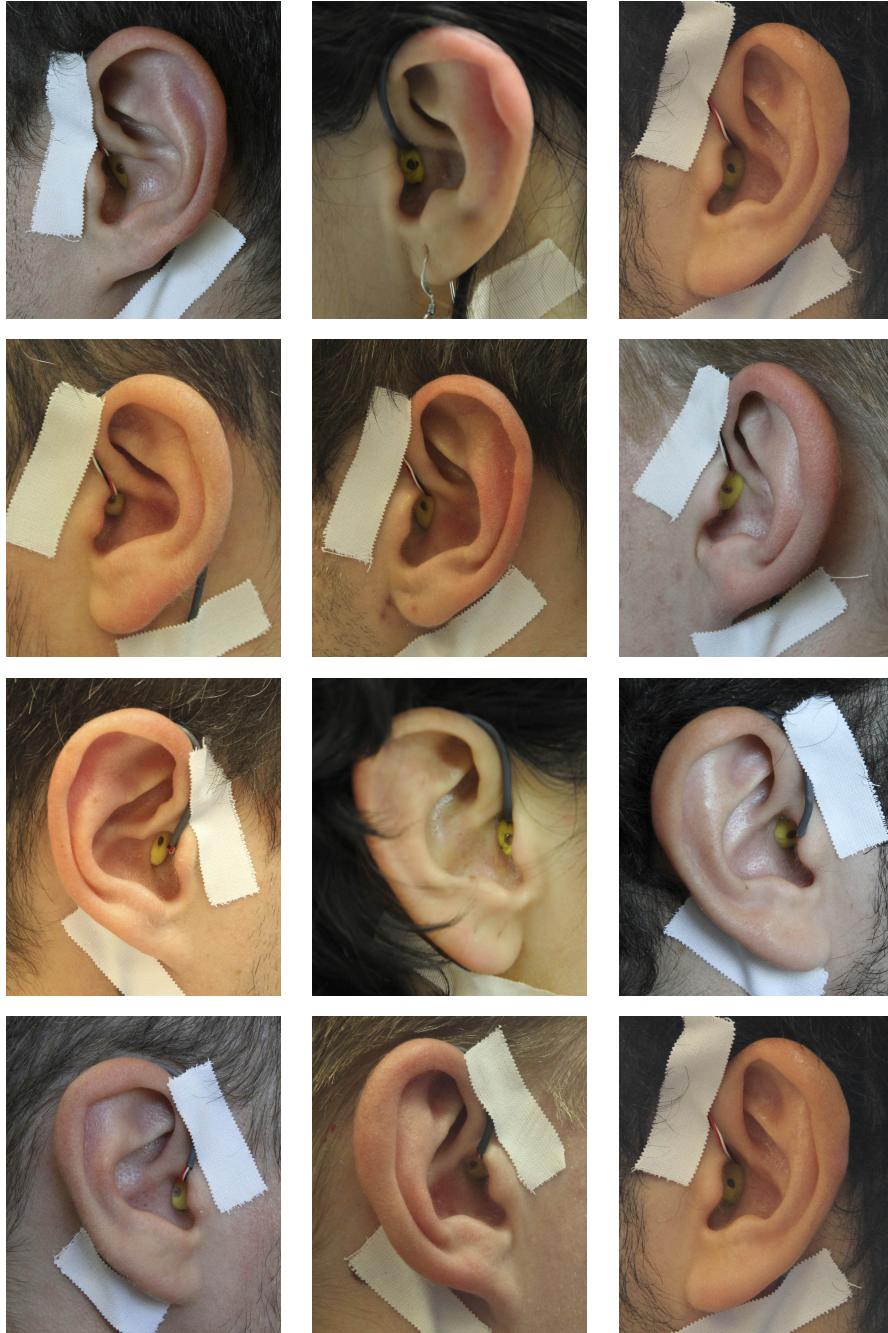
Figure 4.6. Examples of pinnae with microphones in blocked ear canal condition
