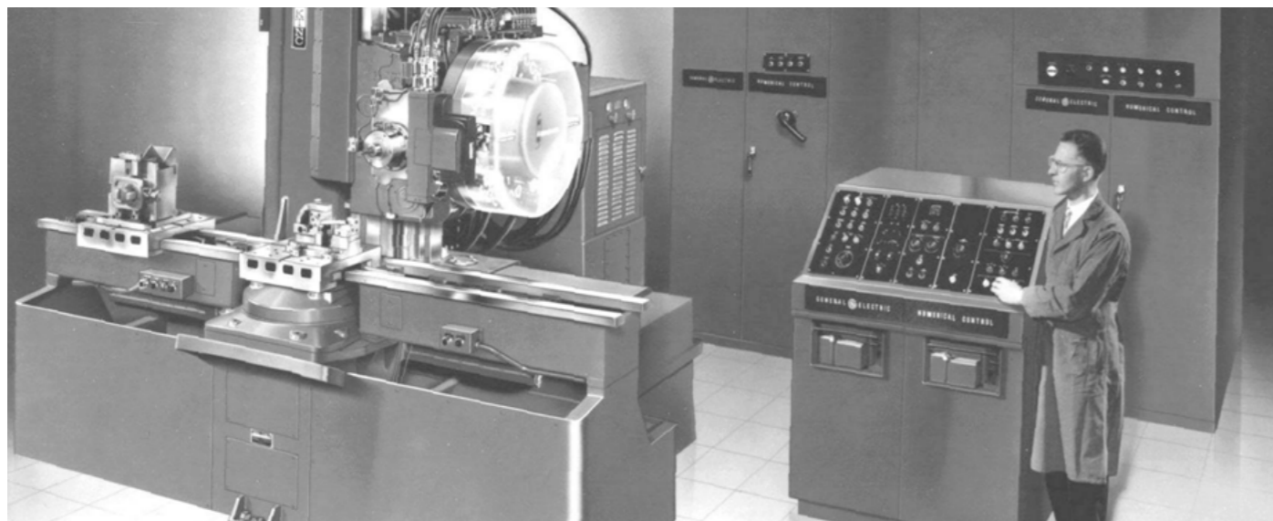
Fig. 4.2 First Control Numerical Machine developed by Parsons [18].
