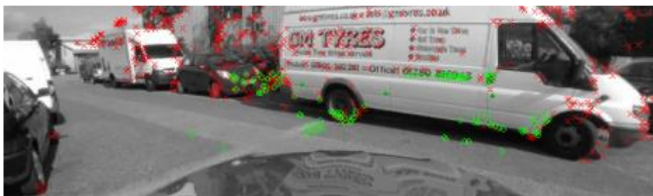
Figure 5-8 Part of a frame corresponding to the part highlighted in green in Figure 5-7 at video time 180 sec, where road corners are represented in green.
