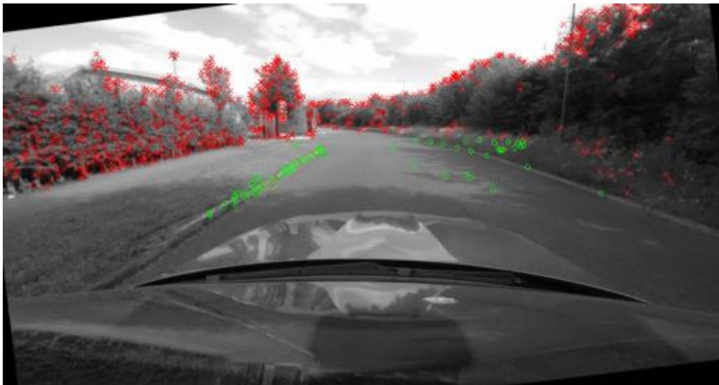
Figure 4-12 Example of a plane fitted to a cloud of points corresponding to the 2D road points (in green) of the bottom image). Units are expressed as a multiple of the separations between the two camera poses (1 unit).
