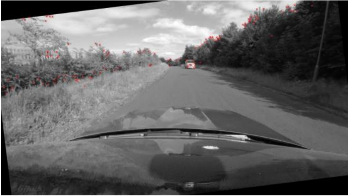
Figure 4-4 Detected corners (red crosses) in a frame of the video with the FAST feature detector configured as follows: Minimum quality = 0.1, Minimum Contrast = 0.2 and ROI = upper half of the image. Total detected corners = 247.
