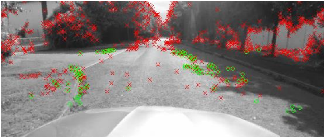
Figure 5-31 Part of a frame corresponding to video section 3 second 245 sec where there are static shadows on the road. Road corners are represented in green.
