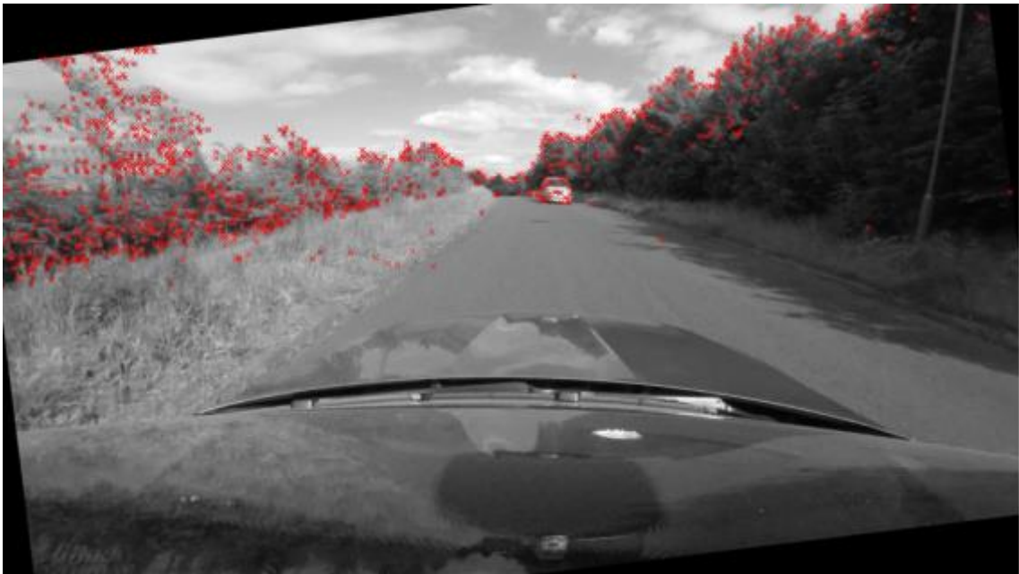
Figure 4-5 Detected corners (red crosses) in a frame of the video with the FAST feature detector configured as follows: Minimum quality = 0.1, Minimum Contrast = 0.2 and ROI = upper half of the image. Total detected corners = 2364.
