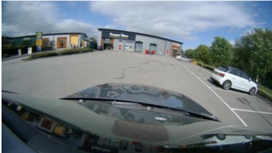
Figure 3-3 Frame from the first seconds of the video. A big barrel distortion caused by the wide-angle lens can be appreciated.
