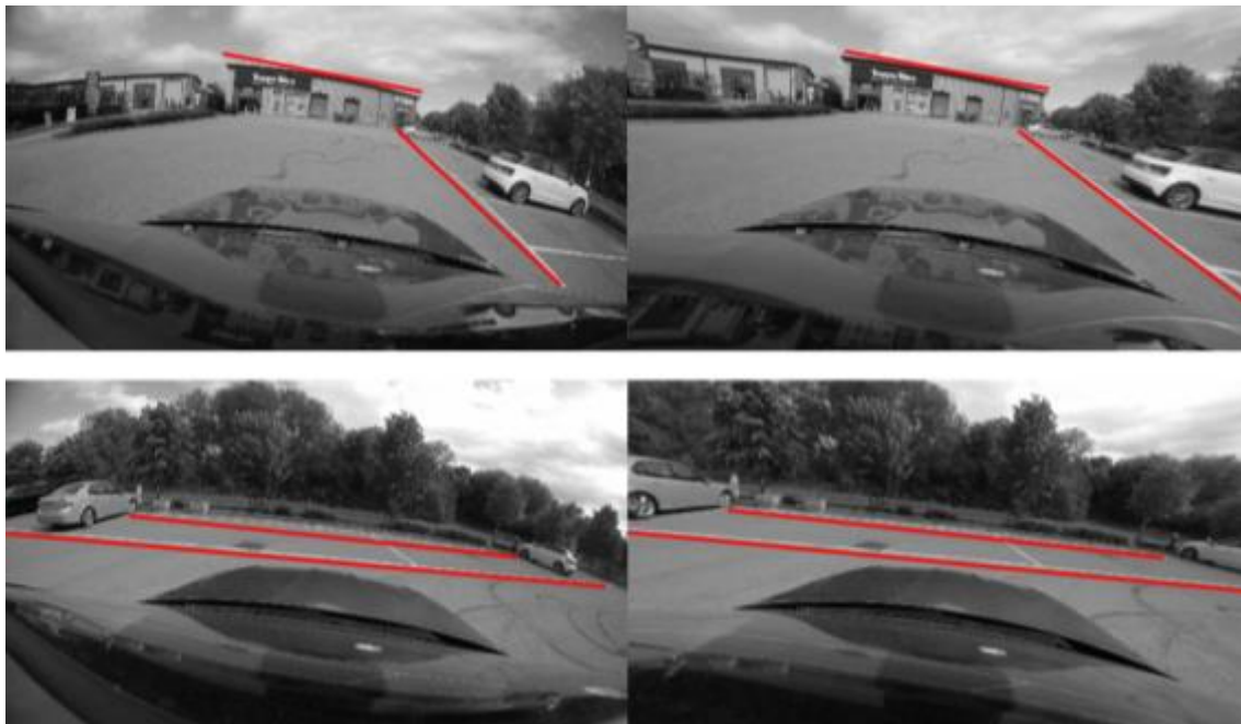
Figure 3-5 Comparison of the original footage (in greyscale) with the images distorted (left images) and the same frames after the lens distortion correction (right images). The red straight lines have been added to these frames to make easier the comparative.
