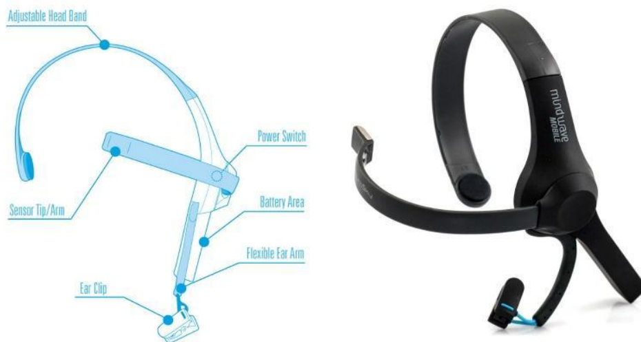
Figure 3.4: Mindwave headset schema
