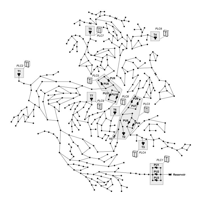
FIG. 1. Graphical representation of C-Town water distribution system (adapted from Taormina et al. 2017).
