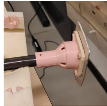
Figure 2.2-2 Redesigned motor support
