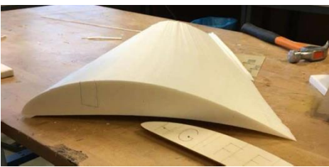
First attempt chambered & tapered wing
