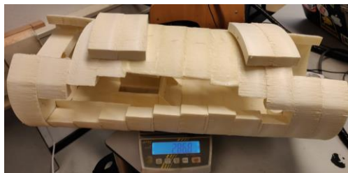
Figure 2.2-3 Assembled fuselage middle
