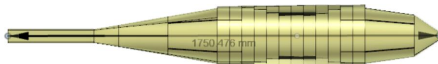
Figure 2-d Total length of the fuselage section
