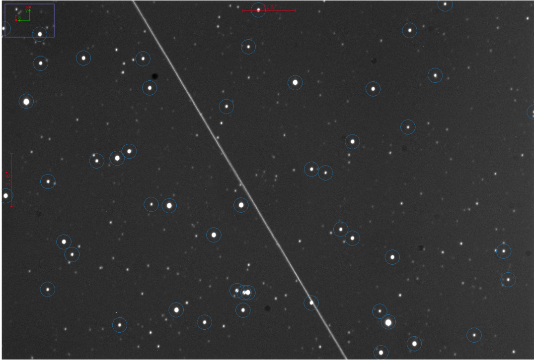
Figure 13: Long exposure image from the UMD Observatory of the pass of the SL-8 rocket body, #7434 of the NORAD catalog.
