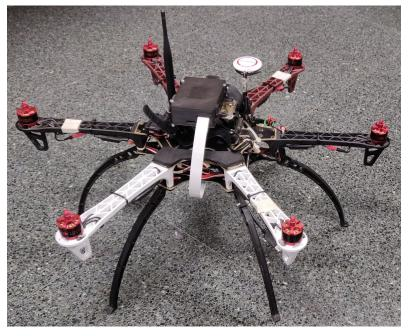
Figure 4. Hexacopter used in our experiments.
