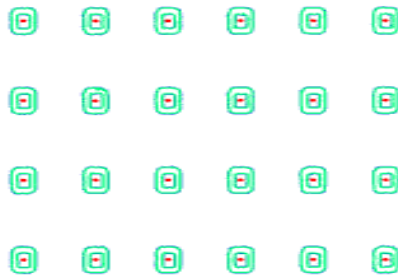
Figure 9 - Pore identification by fitting a binary mask (blue) and their centroids (red)
