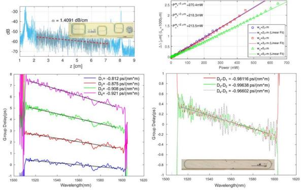
Fig. 1. Spiral waveguide loss measurement (top-left), thermo-optic phase shifter performance (top-right), RR cummulative group delay (bottom-left) and difference (bottom-right).
