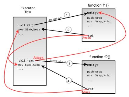
**Figure 2.** Coarse-grained CFI approach bypass example. The attacker is able to redirect the control flow from multiple call()s and ret points. Arrows in red show the valid destinations where attackers can redirect the flow.
