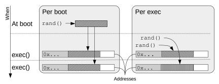
Figure 1. Per-boot versus Per-exec randomization.
