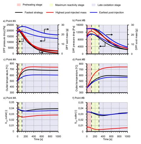
**Figure 13.** DPF pressure drop, soot mass, outlet temperature and outlet O<sub>2</sub> concentration during the fastest active regeneration, advancing the post-injection and increasing the post-injected fuel mass rate.
