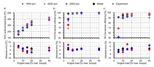
**Figure 3.** Comparison between experimental and modelled results under steady-state conditions of (a) DOC outlet gas temperature, (b) CO conversion efficiency and (c) hydrocarbons (HC) conversion efficiency.
