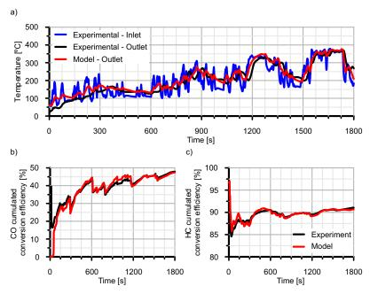
**Figure 4.** Comparison between experimental and modelled results under Worldwide harmonized Light duty Test Cycle (WLTC) conditions of (a) DOC outlet gas temperature, (b) CO conversion efficiency and (c) HC conversion efficiency.
