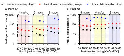
Figure 14. Post-injected fuel mass consumption to complete each regeneration stage.
