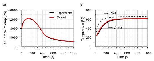
**Figure 5.** Comparison of experimental and modelled results during an active DPF regeneration event of (a) DPF pressure drop and (b) DPF gas temperature.
