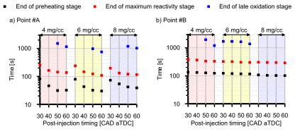
**Figure 12.** Effect of the variation of the post-injection timing and fuel mass on the duration of each regeneration stage.
