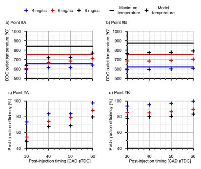
**Figure 10.** Post-injection efficiency as a function of the post-injection timing and the post-injected fuel mass rate.
