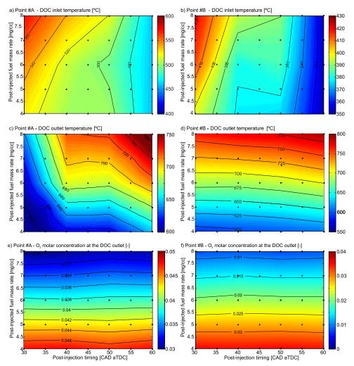
**Figure 9.** Effect of the post-injection timing and the post-injected fuel mass rate on the DOC gas temperature and the O<sub>2</sub> concentration at the DOC outlet.
