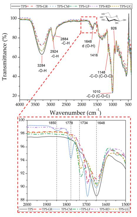
**Figure 7.** Fourier transform infrared spectroscopy (FTIR) spectra with representative peaks of net TPS and its comparison with TPS-resin blend formulations. A zoom in the range between 2000 cm<sup>-1</sup> and 1500 cm<sup>-1</sup> is also shown.
