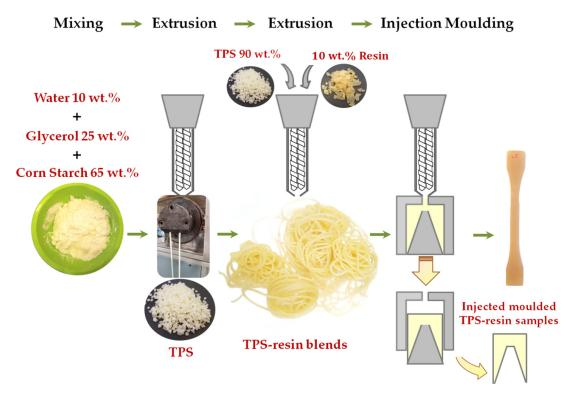
**Figure 2.** Schematic representation of the thermoplastic starch (TPS) preparation and the processing of TPS–resin blend formulations.
