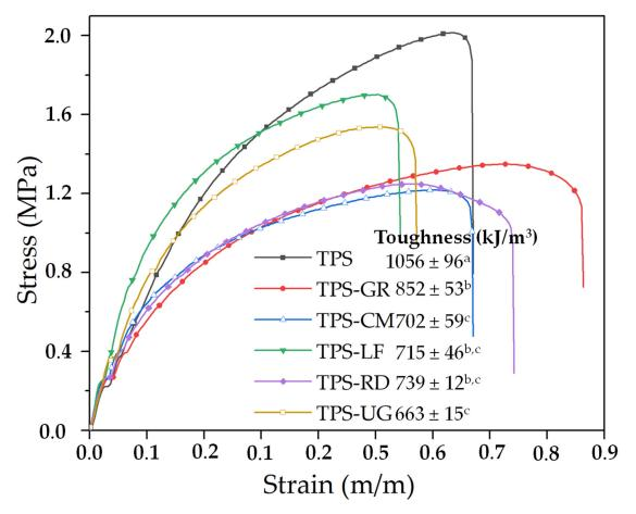
**Figure 4.** Stress–strain curves of TPS and TPS-resin blend formulations with the toughness values. <sup>a–d</sup> Different letters within the same property show statistically significant differences between formulations (p < 0.05).
