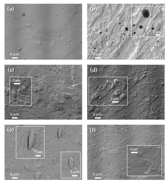
**Figure 8.** Scanning electron microscopy (SEM) images of the crio-fractured surface of: (a) TPS, (b) TPS-GR, (c) TPS-CM, (d) TPS-LF, (e) TPS-RD and (f) TPS-UG.
