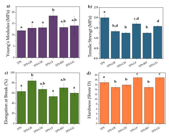
**Figure 3.** Tensile and hardness properties of TPS and TPS-resin formulations: (a) Young modulus, (b) Tensile Strength, (c) elongation at break and (d) Shore D. <sup>a–d</sup> Different letters within the same property show statistically significant differences between formulations (p < 0.05).
