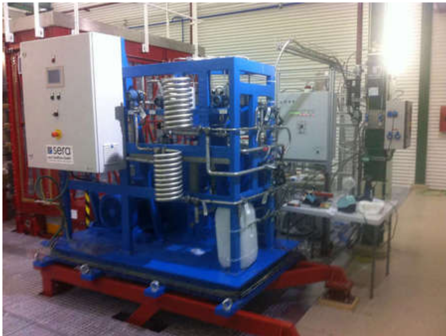
Figure 19: The NEXT-WhiteNEXT-100 compressor, manufactured by SERA.
