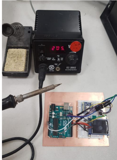
Figure 12: Weller EC2002 hand soldering device
