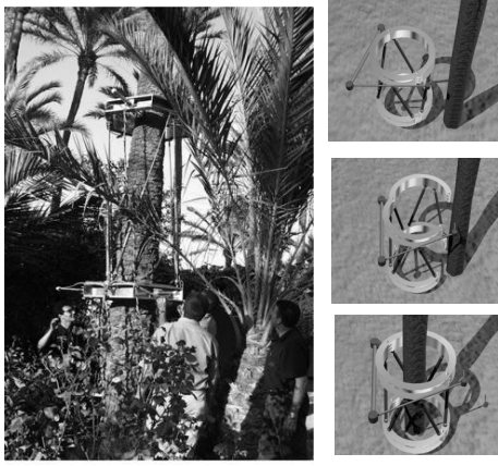
Figura 19. Robot TREPA (UPM-UMH)
