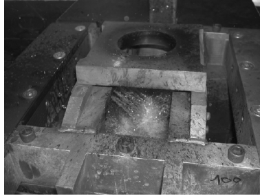
Figure 1.8: Water injection devices used in the experiment of Gély et al. (from [8]).
