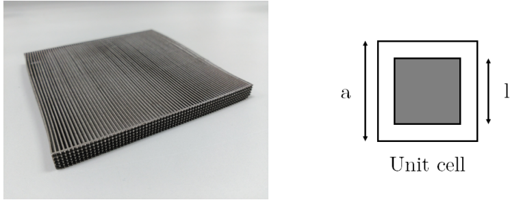
Figure 2.7: 2-D sonic crystal composed by rods of aluminum (left) and scheme of a unit cell (right).
