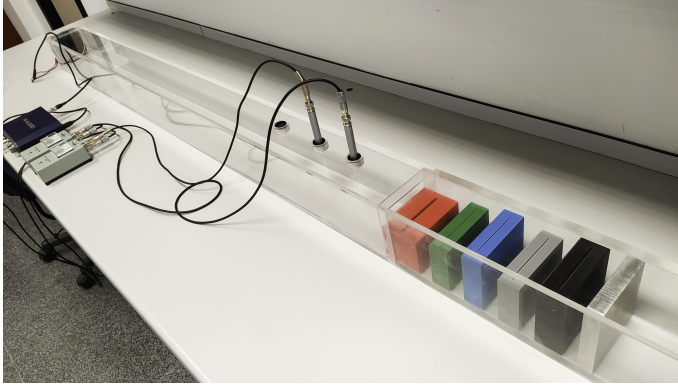
Figure 5.6: Experimental set-up used for the Transfer Function Method.
