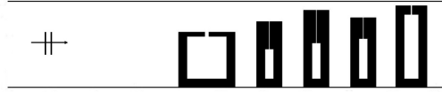
Figure 5.3: Tuned geometry of the optimized system for perfect sound absorption from 400 to 560 Hz.
