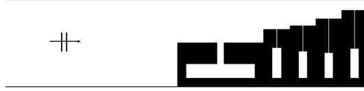
Figure 6.4: Tuned geometry of the optimized system for perfect sound absorption from 400 to 560 Hz with no cavities.
