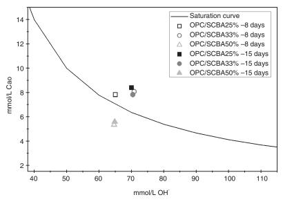
FIGURE 5. Frattini test results for OPC/SCBA pastes after 8 and 15 days.
