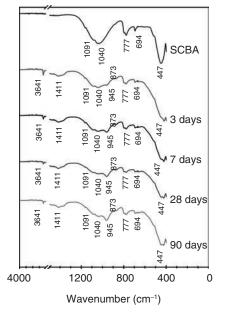
FIGURE 3. FTIR spectra for SCBA and CH/SCBA pastes after 3, 7, 28 and 90 days of curing.
