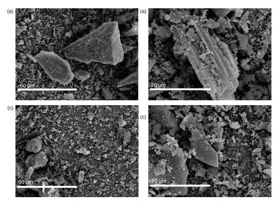
FIGURE 2. SEM images of SCBA: a) and b) before milling process; c) and d) after a milling time of 50 minutes.
