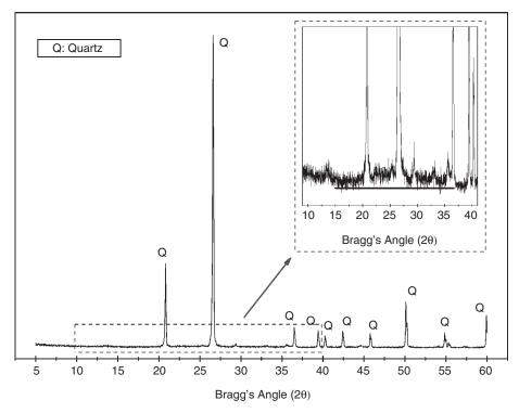
FIGURE 1. X-Ray Diffraction pattern of the SCBA.
