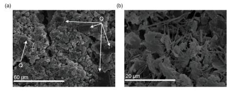
FIGURE 6. SEM images of CH/SCBA pastes after 90 days of curing (Key: Q, quartz).
