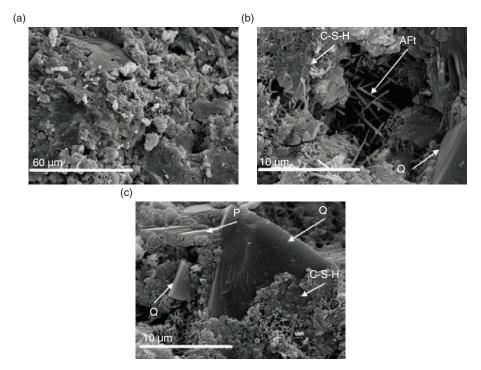
FIGURE 7. SEM images of OPC/SCBA pastes after 28 days of curing (Keys: Q, quartz; P, portlandite; C-S-H, calcium silicate hydrate; AFt, ettringite).
