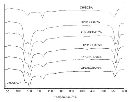
FIGURE 4. DTG curves for CH/SCBA and OPC/SCBA pastes after 90 days of curing.
