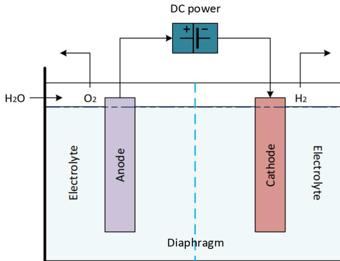
**Figure 3.11:** Electrolysis cell diagram
