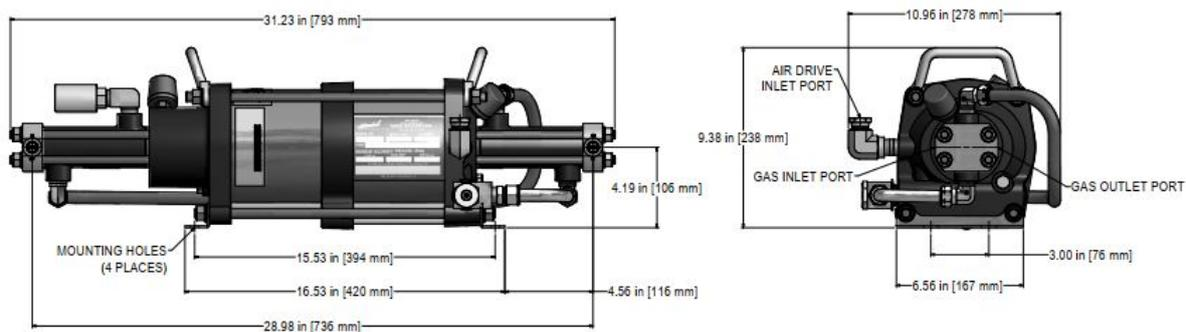
**Figure C.6:** Pneumatic Driven Gas Booster Dimensional Drawings. Gas Boosters Models: AGD-32, AGD-62, AGD-102, AGD-152 [HASKEL, no date]
