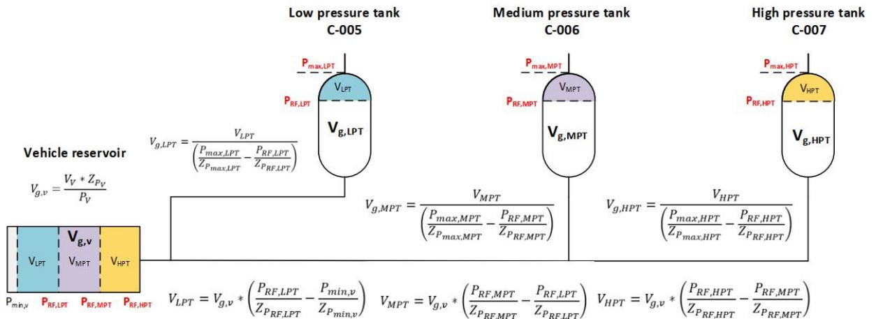
Figure 5.18: Calculation procedure for the hydrogen cascade storage system (450 bar)
