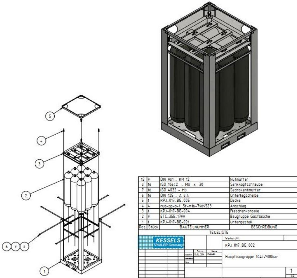
Figure C.3: 900 bar storage tank system technical drawing. Model KPJ-017-BG-002 [NPROXX, no date]
