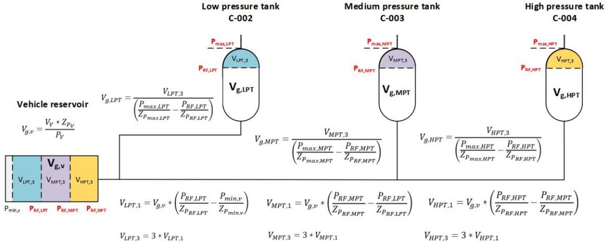
**Figure 5.15:** Calculation procedure for the hydrogen cascade storage system (900 bar)
