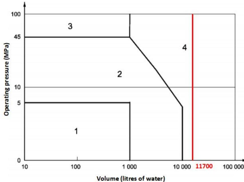
**Figure 5.3:** Classification of hydrogen gas storage to determine safety distances [ISO/TS 20100, 2008]
