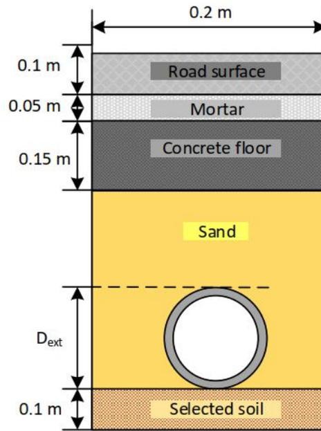
**Figure 5.37:** Construction detail of the hydrogen pipes trench
