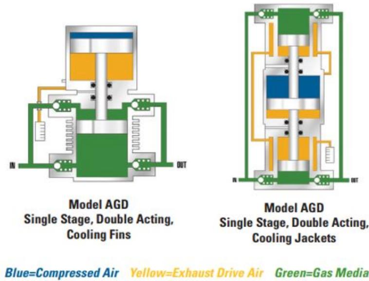
**Figure 5.21:** AGD Pneumatic Driven Gas Booster Configurations [HASKEL, no date]
