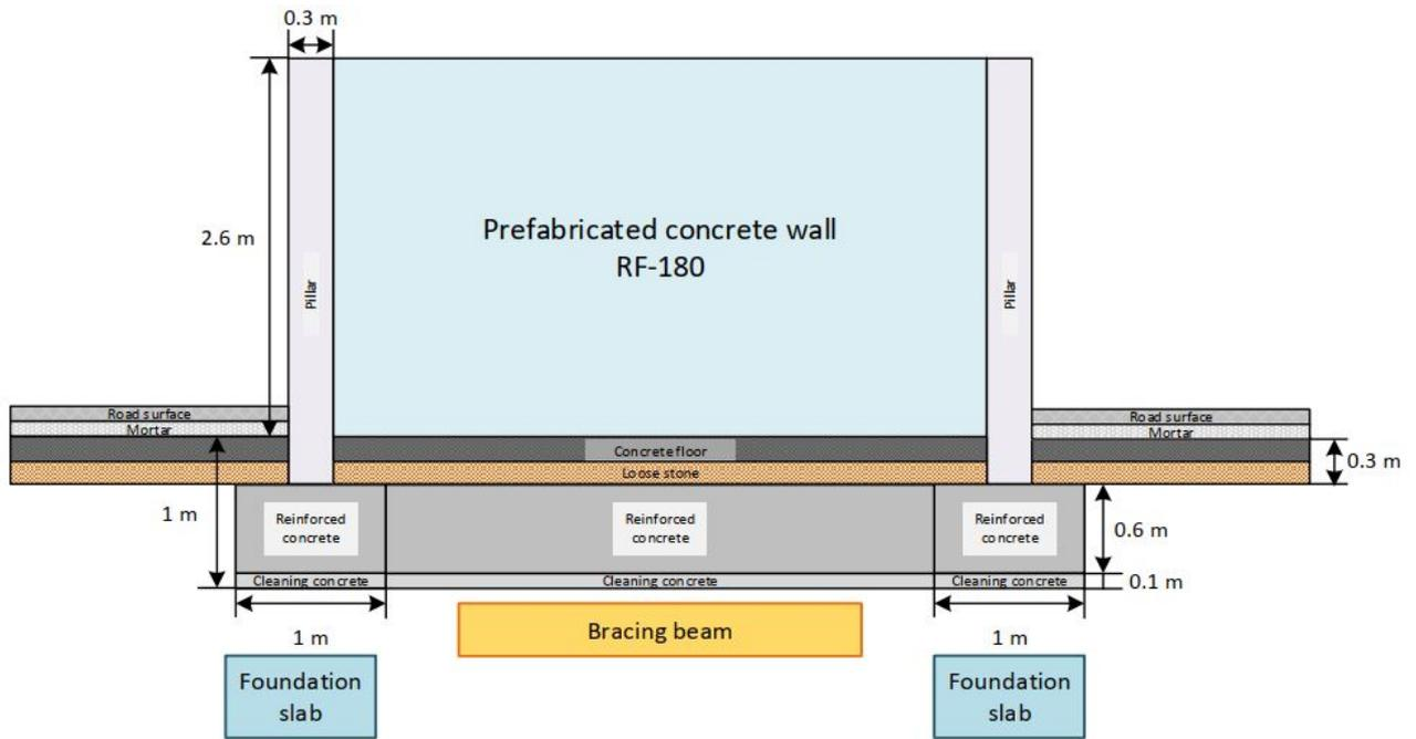
**Figure 5.35:** Construction detail of the Engine Rooms trench
