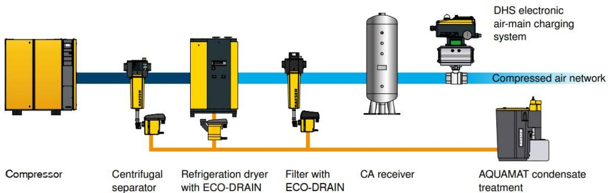
**Figure 5.46:** Air compressor system components [KAESER COMPRESSORS AC, no date]
