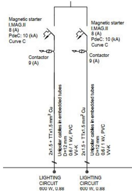
**Figure 5.39:** One line electric diagram for the lighting circuit
