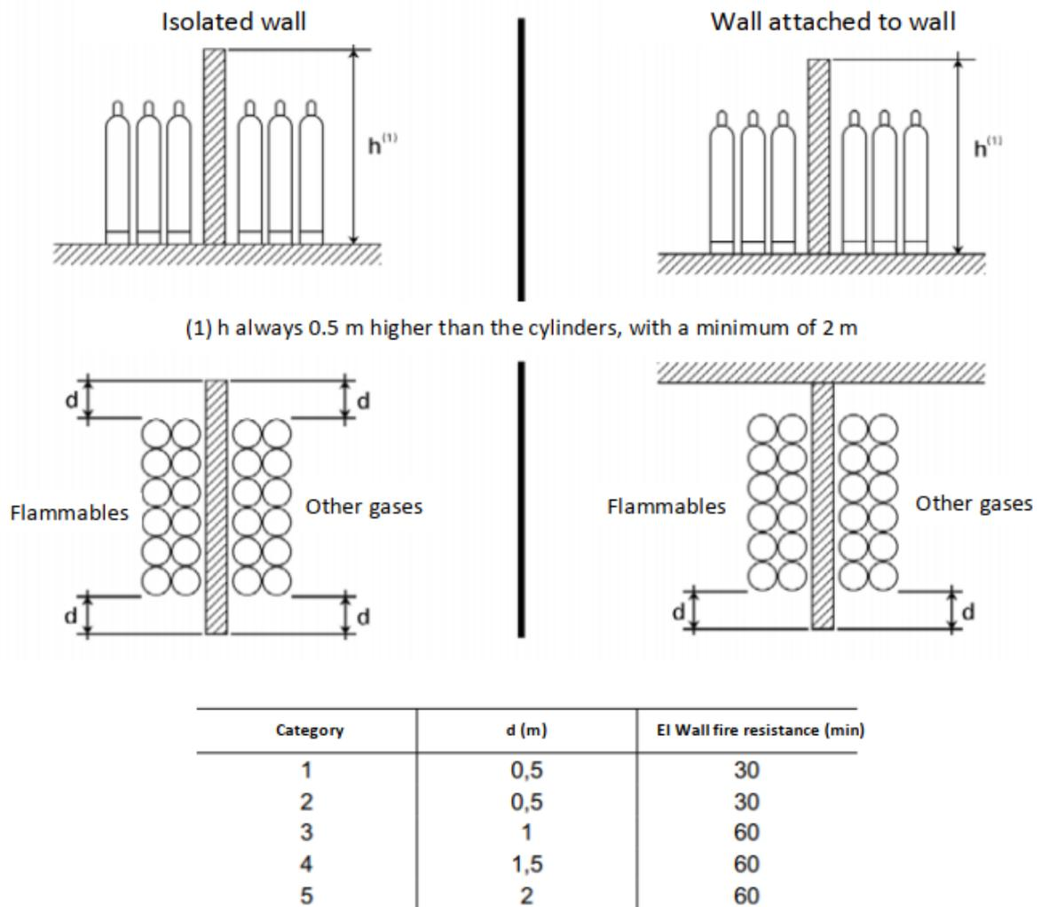
**Figure B.5:** Separation between cylinders of flammable and other gases (With separation wall). ITC MIE-APQ 5 (RD 656/2017)
