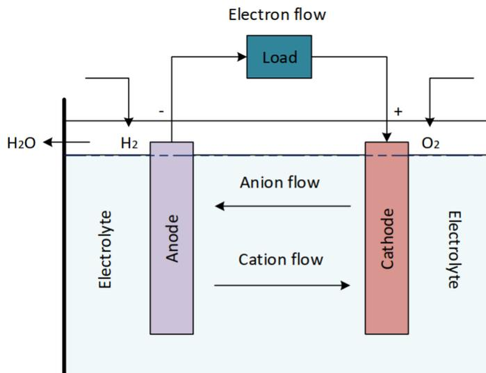
**Figure 3.4:** Fuel cell diagram
