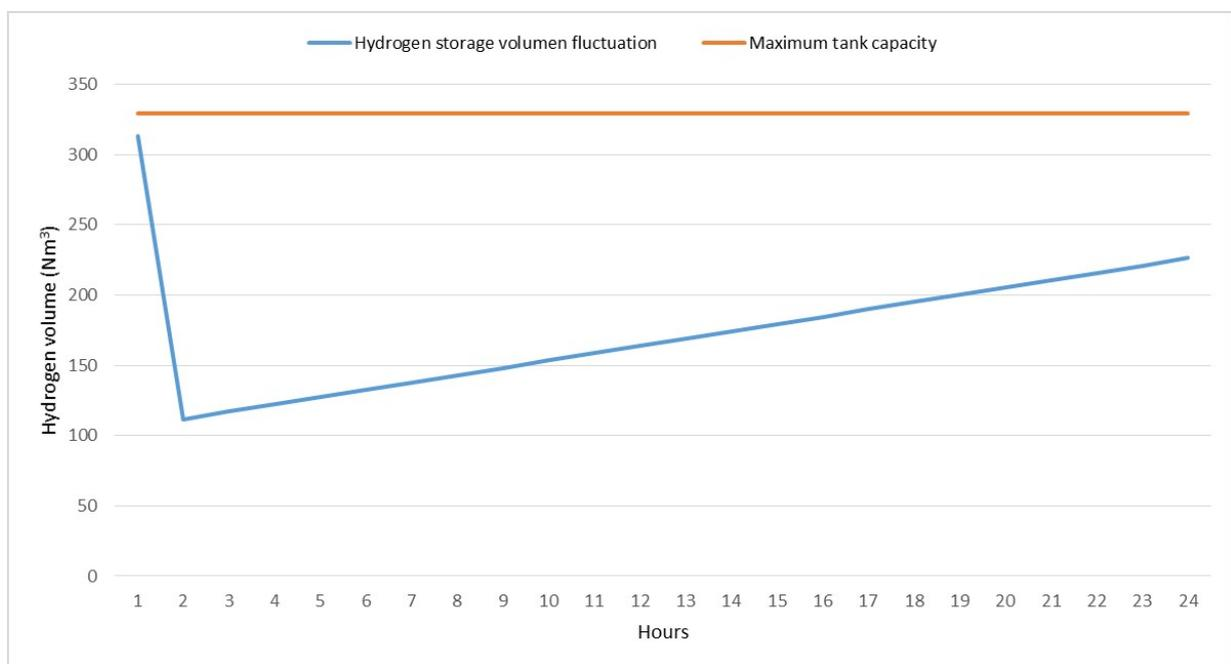
**Figure 5.11:** Hydrogen storage fluctuation ( $\text{Nm}^3 \text{ H}_2$ ) in the low pressure tank (Day 1)
