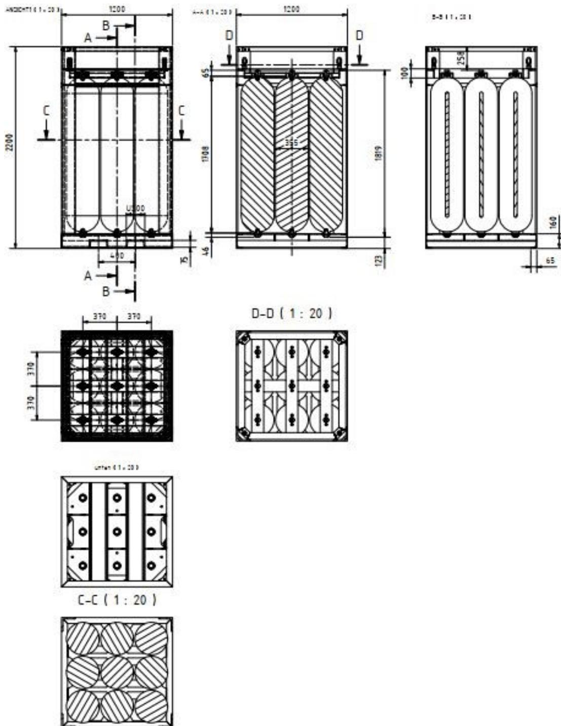
**Figure C.4:** 900 bar storage tank system technical drawing (views and dimensions). Model KPJ-017-BG-002 [NPROXX, no date]
