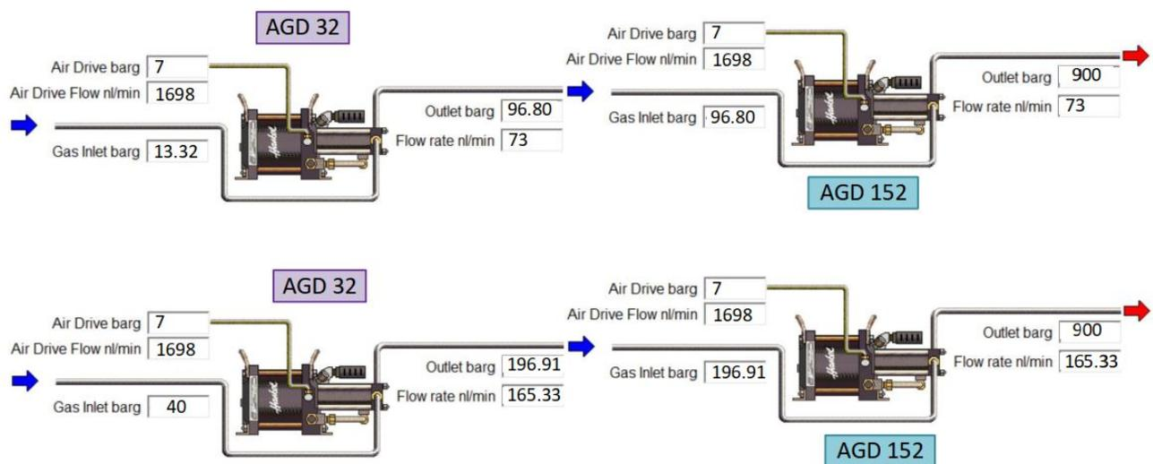
**Figure 5.23:** AGD Boosters series connection simulations (900 bar line). Minimum supply pressure (top) and maximum supply pressure (bottom) [HASKEL, no date]
