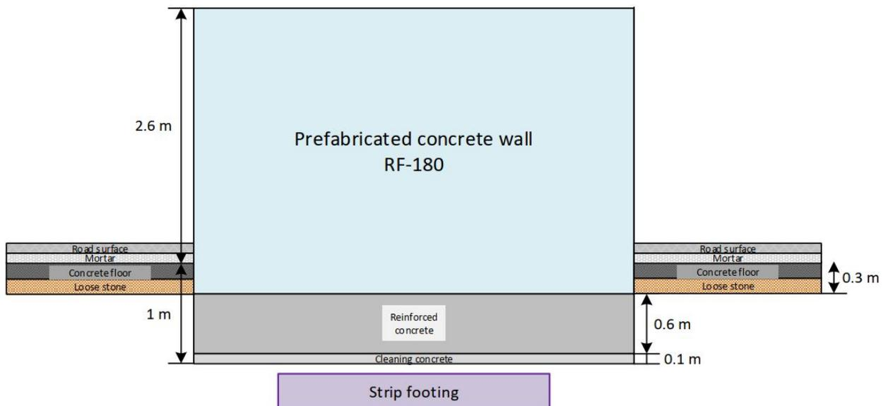
**Figure 5.36:** Construction detail of the walls trench
