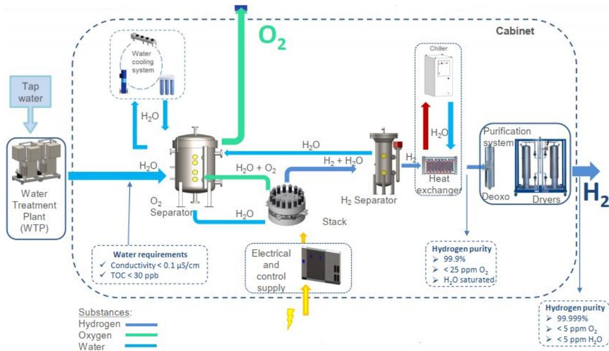
Figure 5.7: General scheme of the electrolyser [H2B2, no date]
