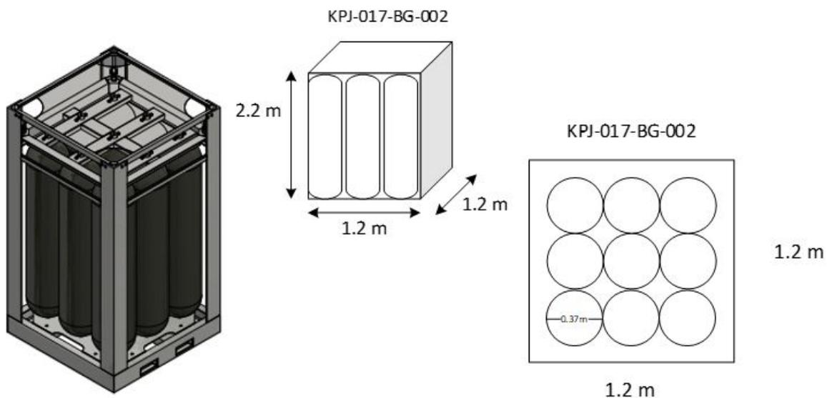
**Figure 5.17:** High pressure storage tank and dimensional views for cascade storage system (900 bar) [NPROXX, no date]
