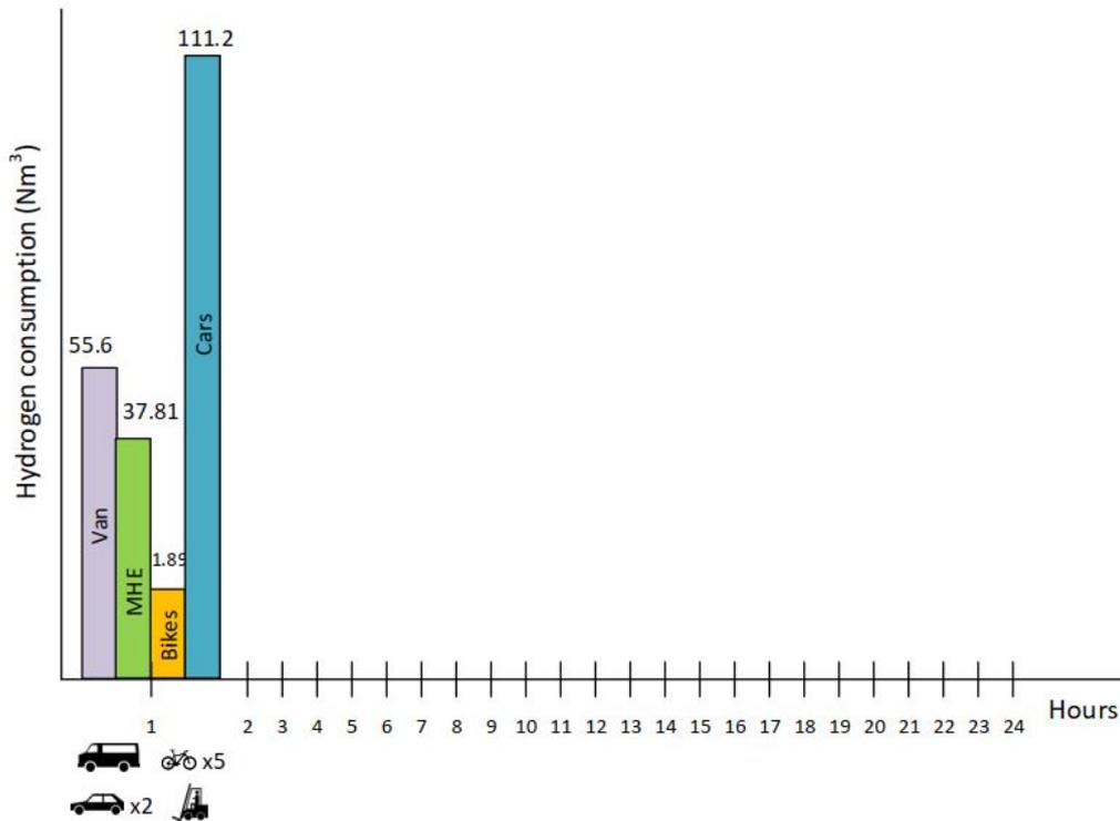
Figure 5.9: Vehicles hydrogen consumption (Day 1)
