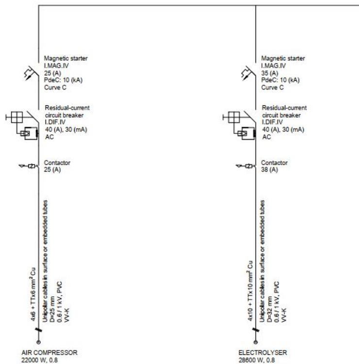
**Figure 5.38:** One line electric diagram for the electrolyser and the compressed air system
