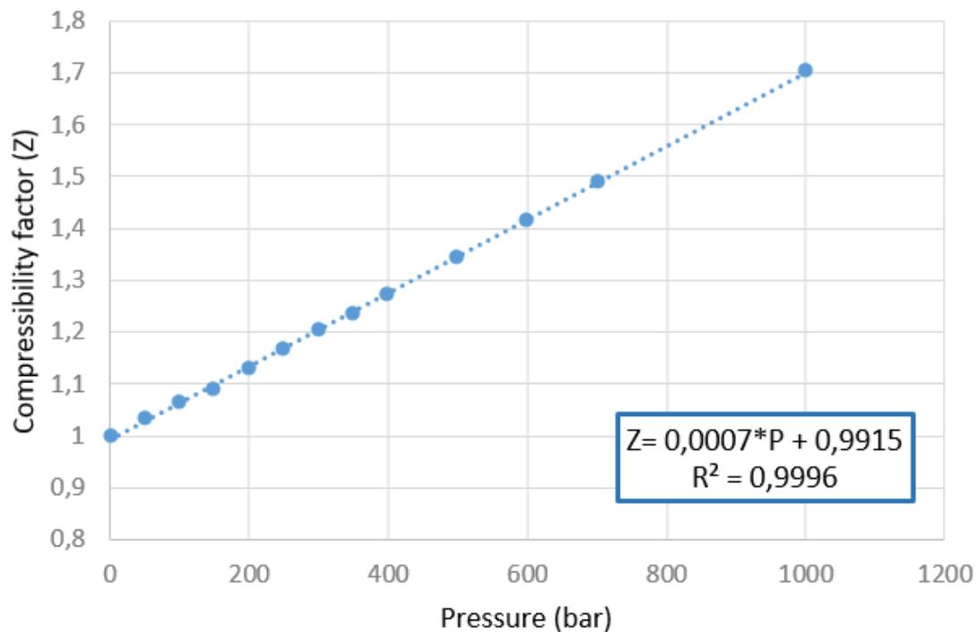
Figure A.4: Linear adjustment of the compressibility factor as a function of pressure
