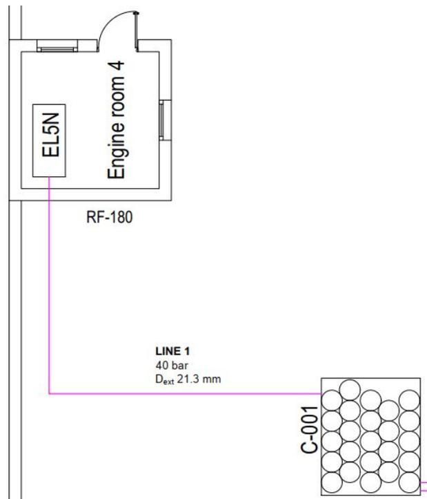
**Figure 5.29:** Hydrogen installation. Line 1
