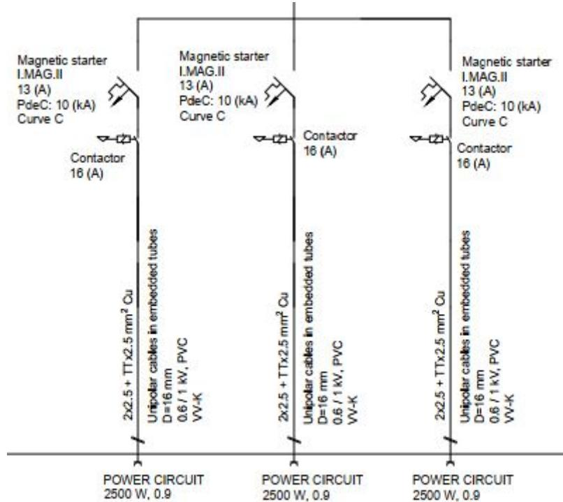
**Figure 5.40:** One line electric diagram for the power circuit
