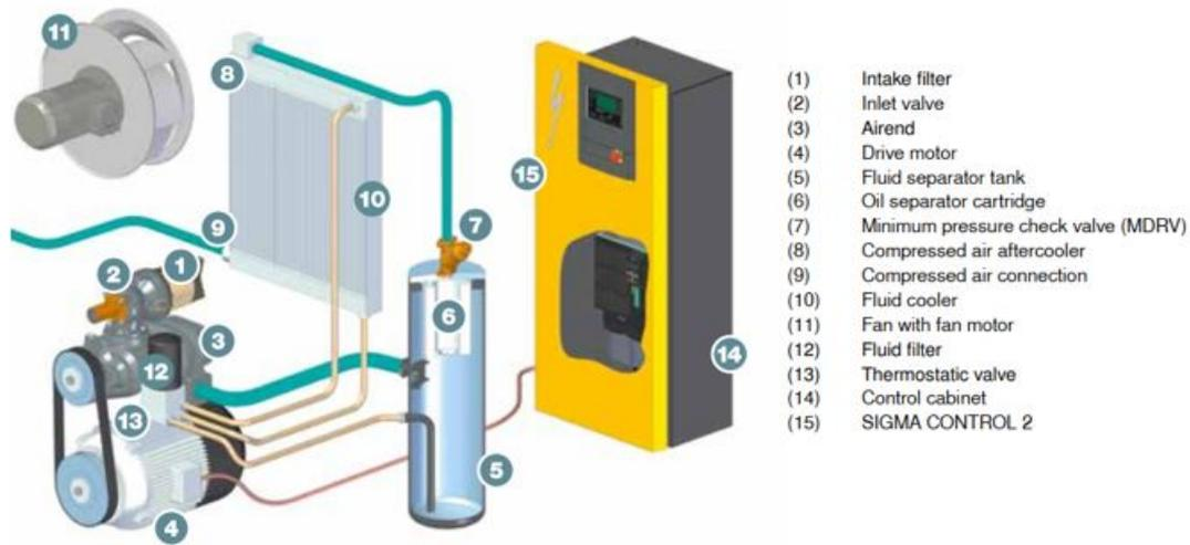
**Figure 5.25:** Air screw compressor working [KAESER COMPRESSORS AC, no date]
