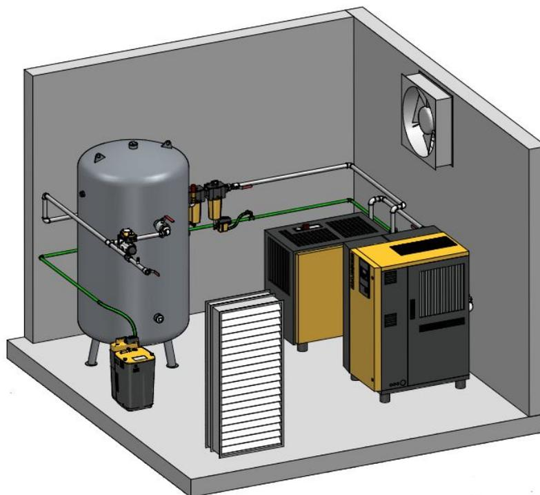
Figure 5.47: Air compressor system layout [KAESER COMPRESSORS AC, no date]
