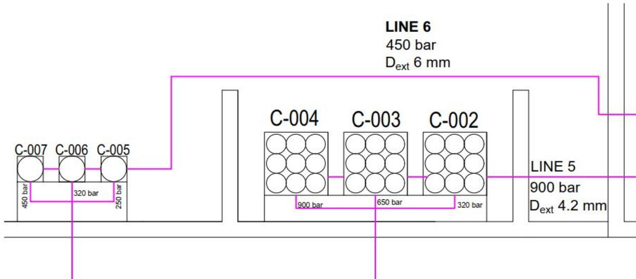
Figure 5.32: Hydrogen installation. Line 5 and line 6
