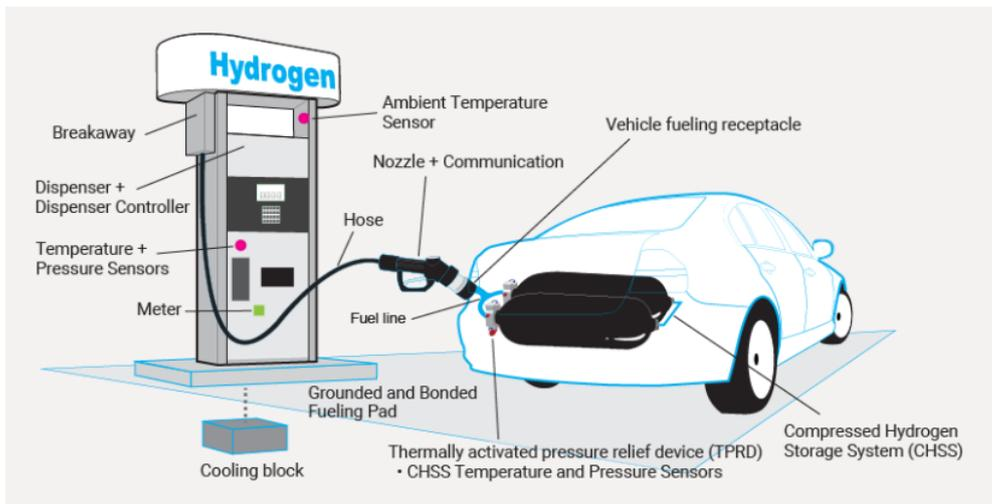
**Figure 3.15:** HRS main components [ISO 19880-1, 2020]
