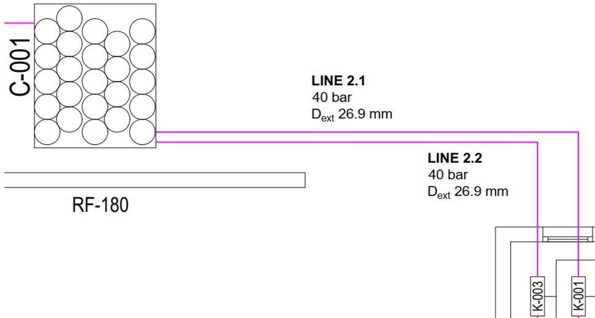
**Figure 5.30:** Hydrogen installation. Line 2.1 and line 2.2
