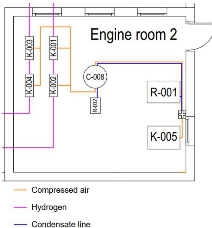
Figure 5.48: Air compressor system technical view
