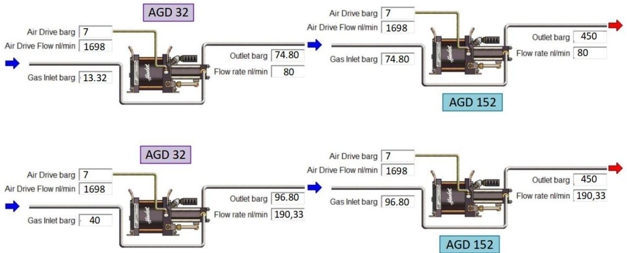
**Figure 5.24:** AGD Boosters series connection simulations (450 bar line). Minimum supply pressure (top) and maximum supply pressure (bottom) [HASKEL, no date]
