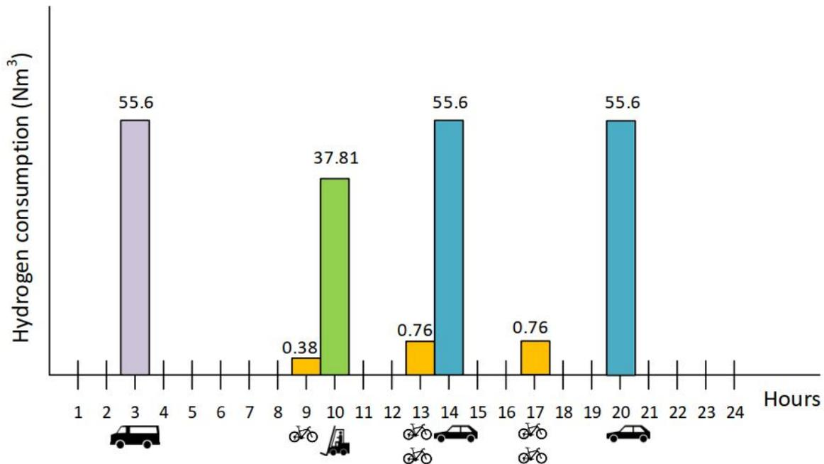
**Figure 5.10:** Vehicles hydrogen consumption (Day 2)
