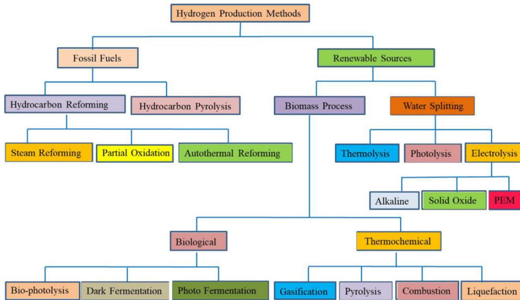
**Figure 3.10:** Hydrogen production methods classification [Shiva Kumar and Himabindu, 2019]
