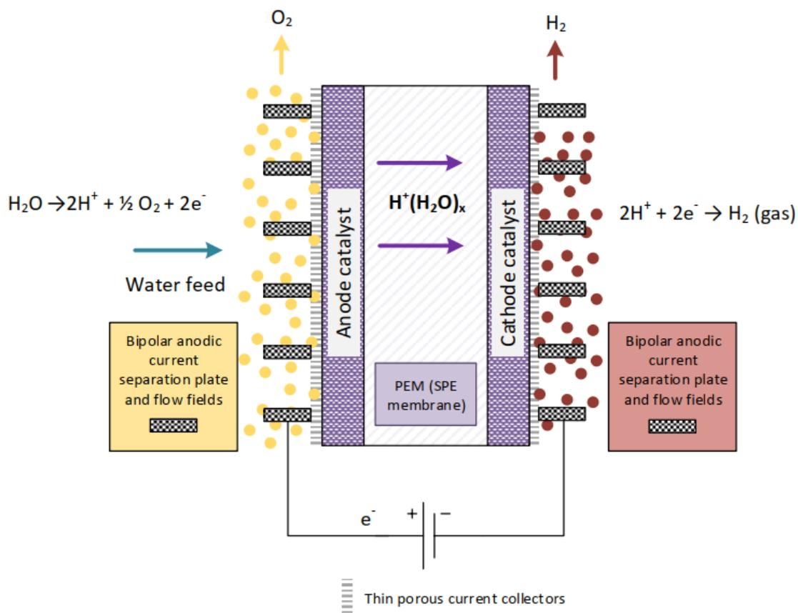
**Figure 3.13:** PEM cell diagram [Bessarabov and Millet, 2018]
