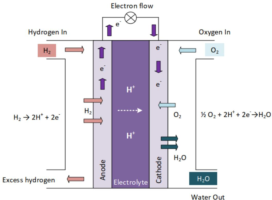
Figure 3.5: PEMFC diagram
