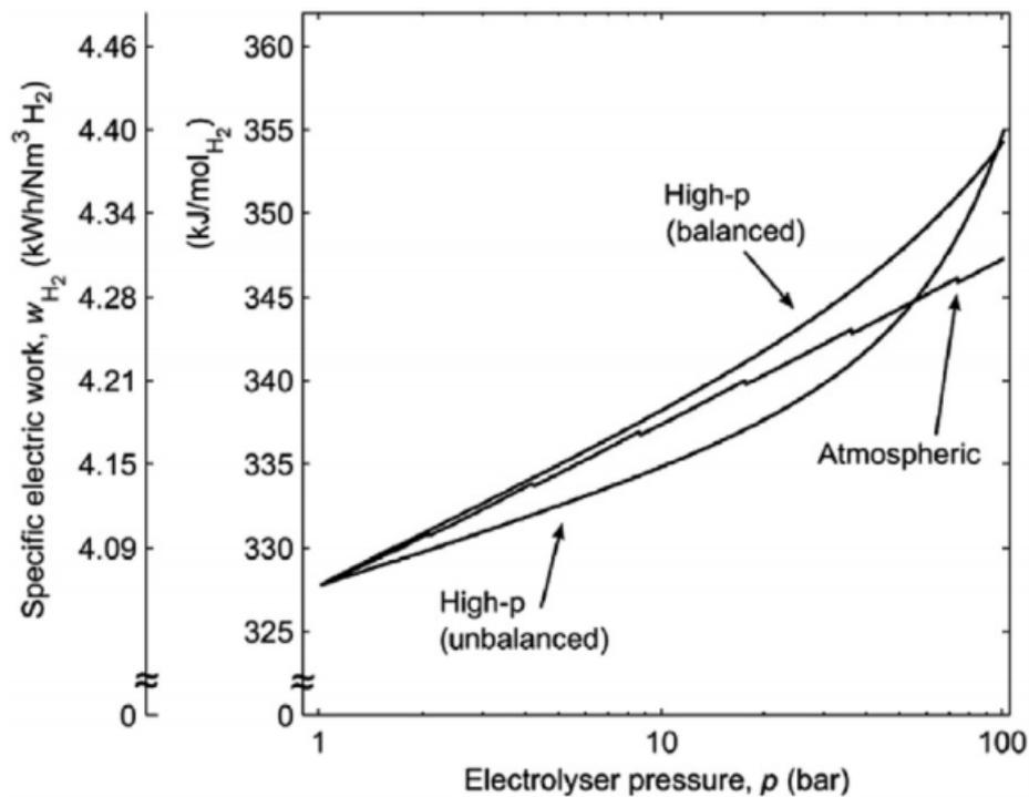
Figure 3.14: Specific energy demand to produce high-pressure hydrogen at 60 °C [Bessarabov and Millet, 2018]
