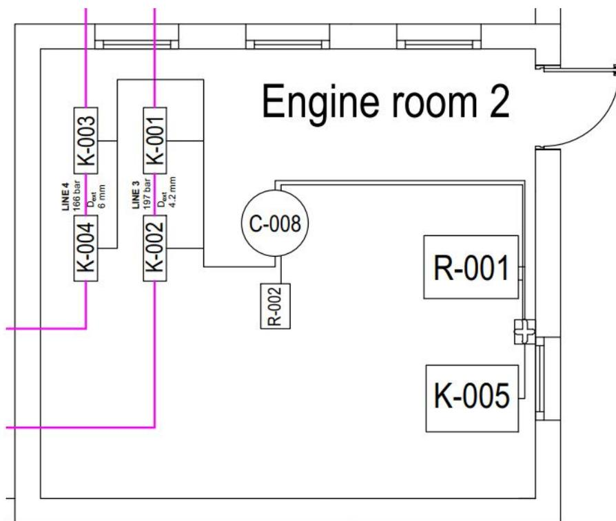
**Figure 5.31:** Hydrogen installation. Line 3 and line 4
