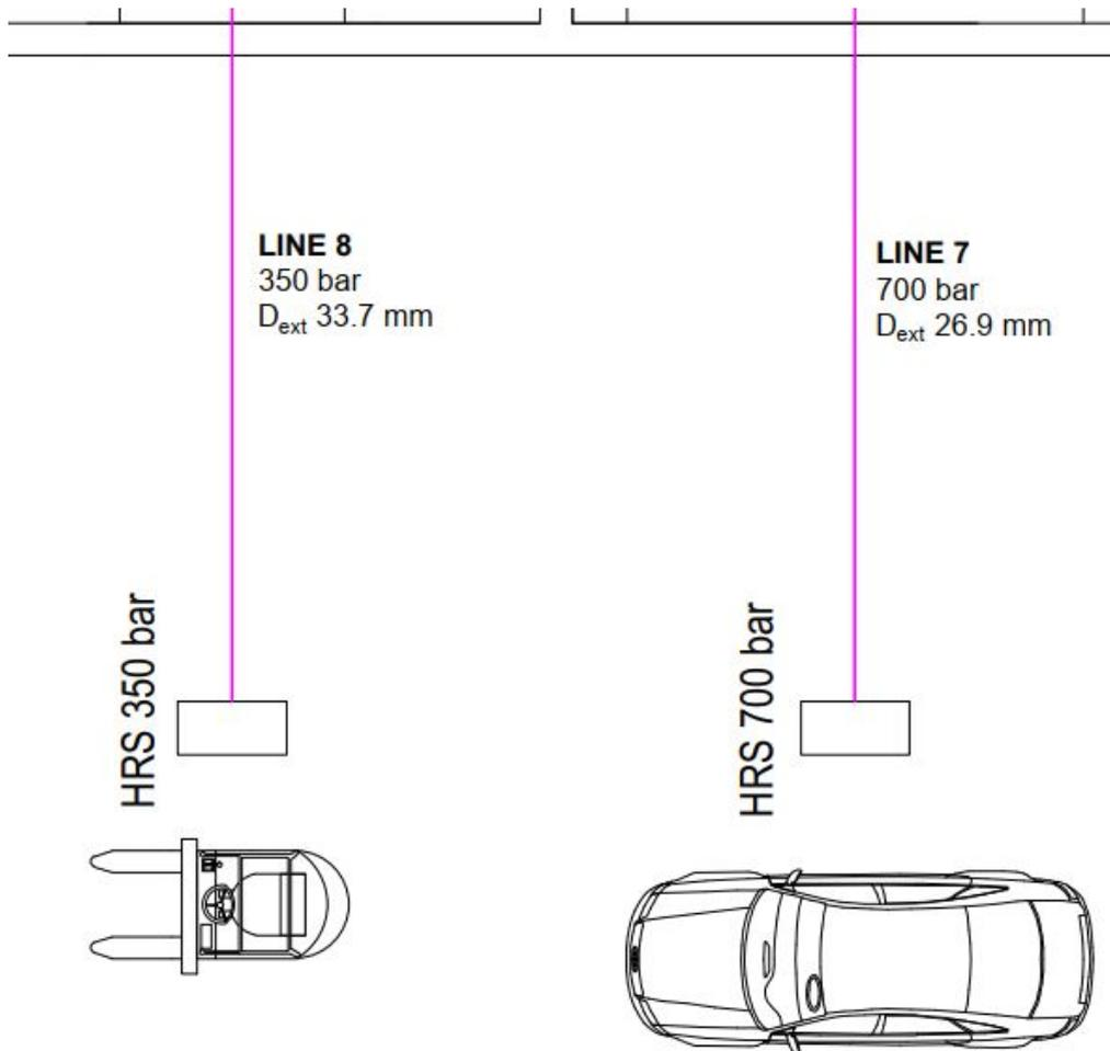
Figure 5.33: Hydrogen installation. Line 7 and line 8
