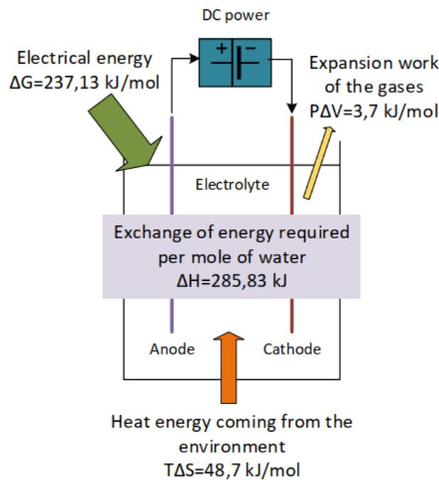
**Figure 3.12:** Energy balance of water electrolysis (1 atm, 298 K) [Llera Sastresa and Zabalza Bribián, 2011]
