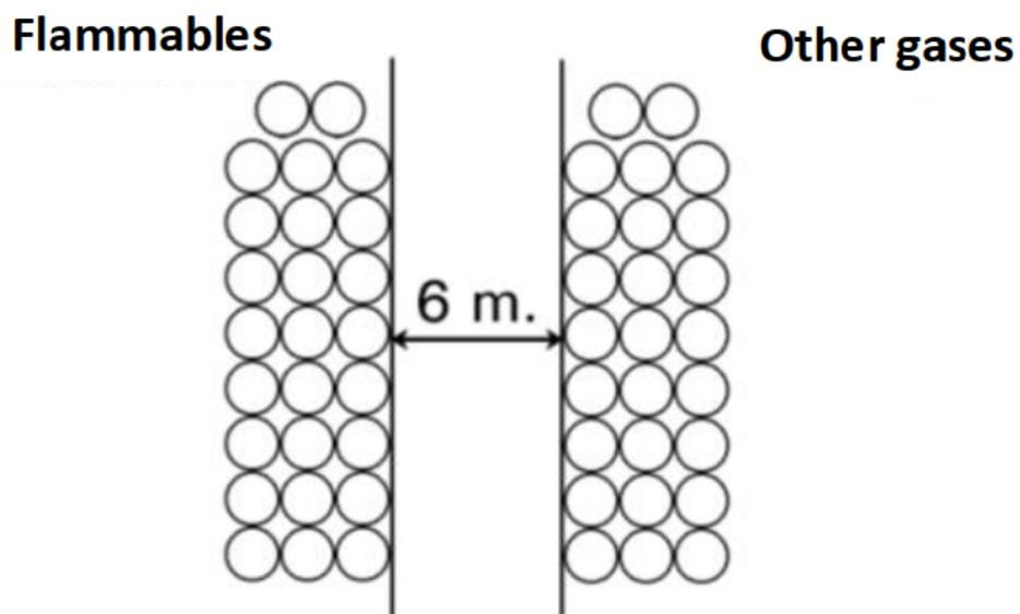
**Figure B.4:** Separation between cylinders of flammable and other gases (Without separation wall). ITC MIE-APQ 5 (RD 656/2017)
