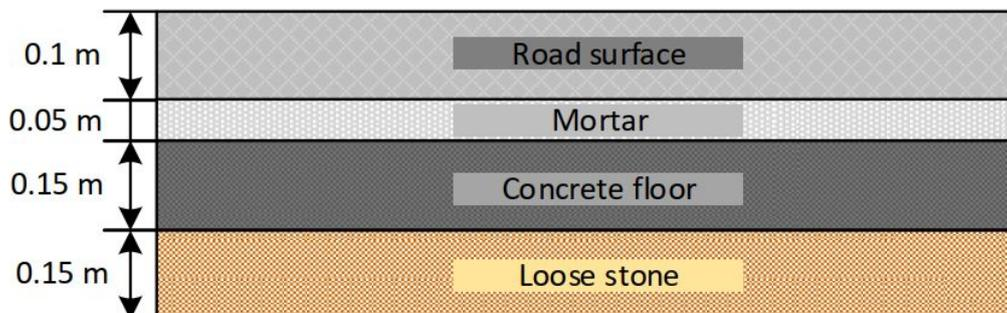
Figure 5.34: Construction detail of the floor trench
