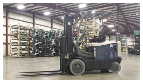
Figure 3.8: Gendrive Series 1000 FCV [PLUG POWER, 2018]
