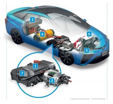
Figure 3.6: Toyota Mirai Fuel Cell Vehicle. Internal components [Toyota, 2015]
