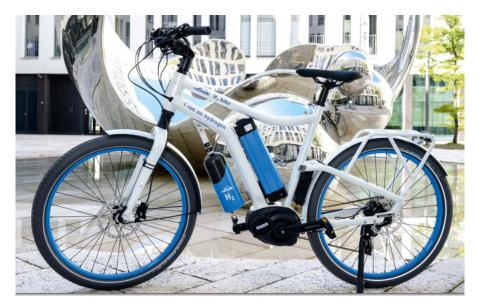
Figure 3.9: Linde  $H_2$  bike [LINDE, no date]
