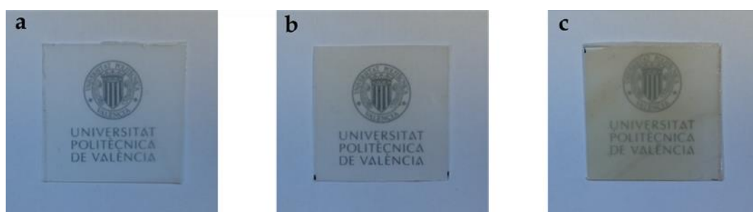
Figure III.4.3.1. Visual appearance of the bio-based high-density polyethylene (bio-HDPE) films containing different amounts of gallic acid (GA): a) Bio-HDPE; b) Bio-HDPE + 0.3GA; c) Bio-HDPE + 0.8GA.
