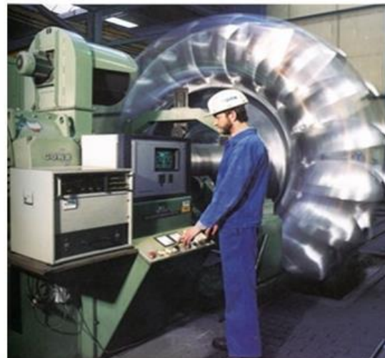
Figure 18 Turbine Pelton- turbine à action.
