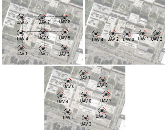
Figure 4.17: Swarm layouts: i) matrix with 9 UAVs, ii) linear with 5 UAVs, and iii) circular with 9 UAVs.
