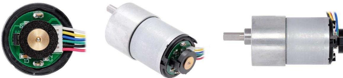
The quadrature encoder provides a resolution of 64 counts per revolution (CPR) of the motor shaft when counting both edges of both channels. To compute the counts per revolution of the gearbox output, multiply the gear ratio by 64.
