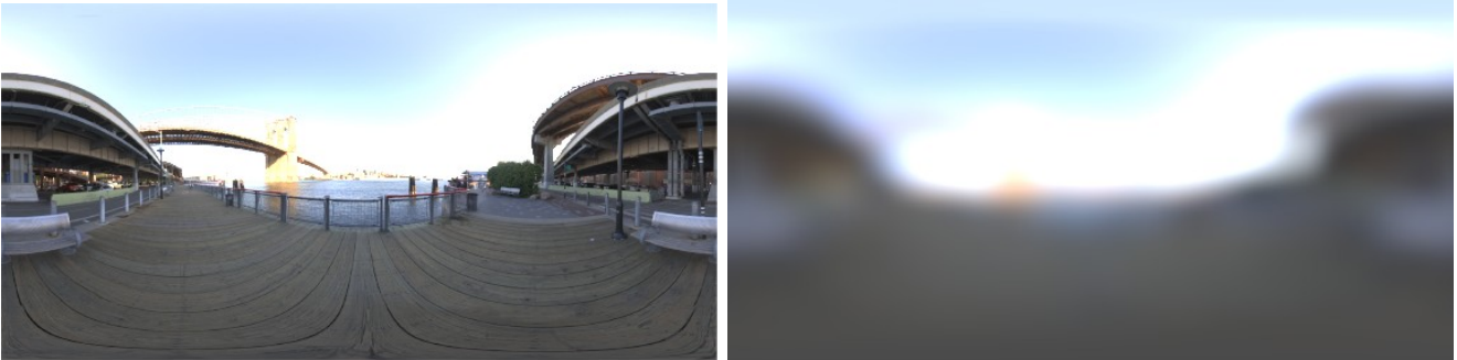
Reflection map vs Diffuse map Example (Refl map: Real resolution: 2048x1024 32bit) (Diff map: Real resolution: 512x256 32bit)
