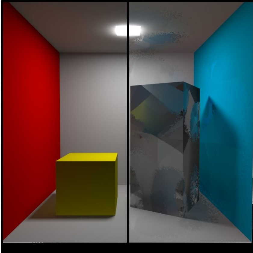
Differences between Low and High quality GI in PointCloud GI calculation. (3Delight Render)
