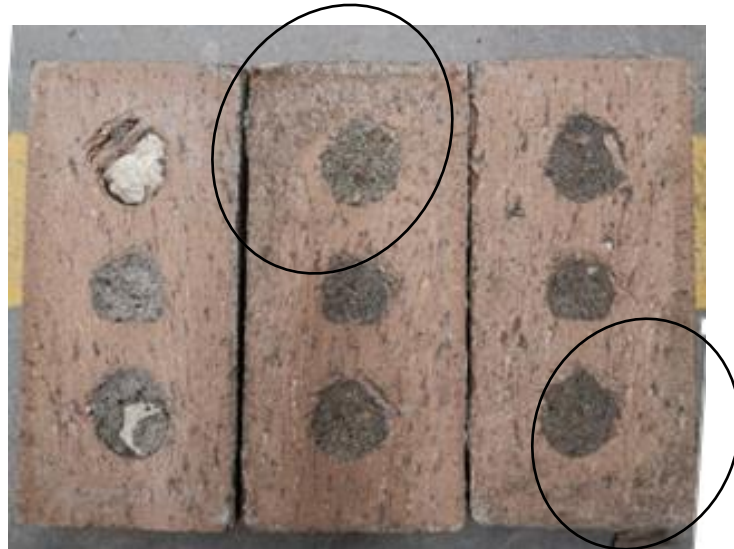
Figure 12. Bricks after bonding test showing sludge particles on the bonding surface (from left to right, M0, M5US, and M5TS)
