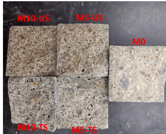
Figure 14. View of the flexural samples after testing, showing the internal structure of the mortar.
