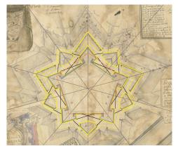
Fig. 4. Auguste de la Vallée, Plan des Sousterrains de la Cittadelle de Turin, 100 trabucchi=147,5 mm (660 x 495 mm). Graphical analysis and geometric construction superimposed on the original plate. (Archivio Storico del Comune, SIM D554. Reconstructive drawing: R. Spallone).
