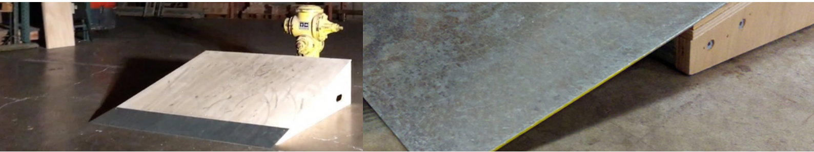
Figura 10: Wedge Bump Ramp.
