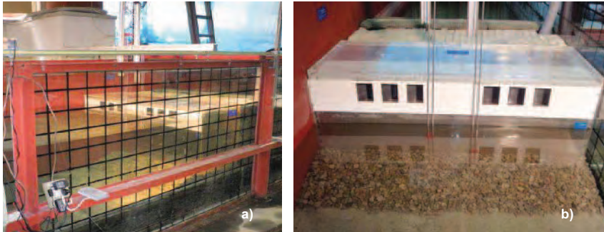
Figure 10: Anti-reflective caisson model in the wave flume (scale 1:35)
