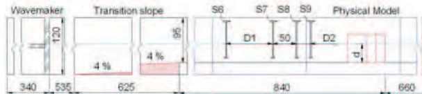
Figure 1. Longitudinal cross section of the LPC-UPV wave flume.
