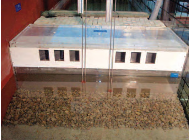
Figure 4.- Front view of new low-reflectivity caisson model (scale 1:35)
