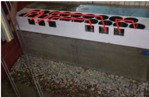
Figure 5.- Low-reflectivity multi-cell circuit caisson model M3
