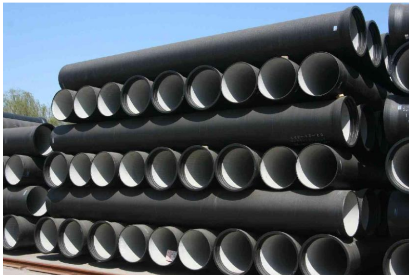
Figure 1 : Ductile cast iron pipes
