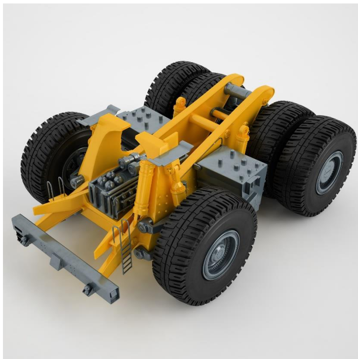
Figure 4 : Haul truck frame with components
