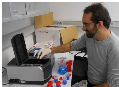
Figure 2.6. Determination of TAN (total ammonia nitrogen, including both the ionized and the un-ionized form) with the T60UV-VIS Spectrophotometer, using the indo-phenol method.
