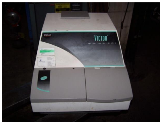
Figure 2.7. Picture of the microplate reader used for nitrate determination.
