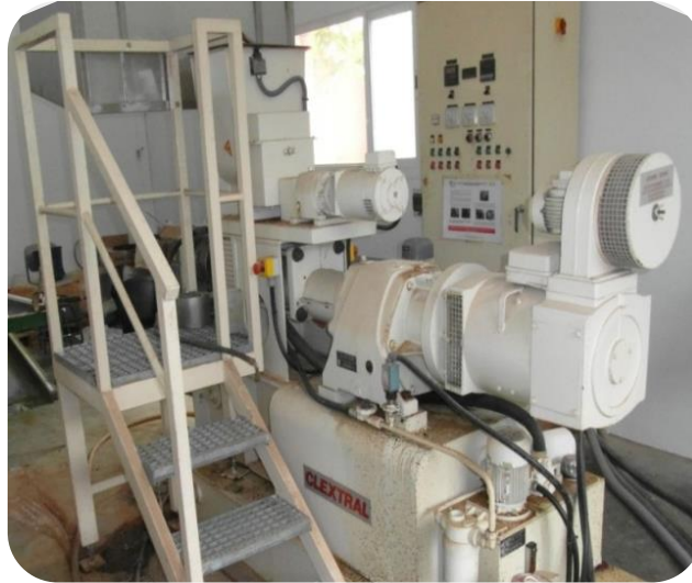
Figure 2.8. Picture of the semi-industrial extruder used to manufacture the experimental diets used in the study in the feed producing laboratory of the Universitat Politècnica de València.
