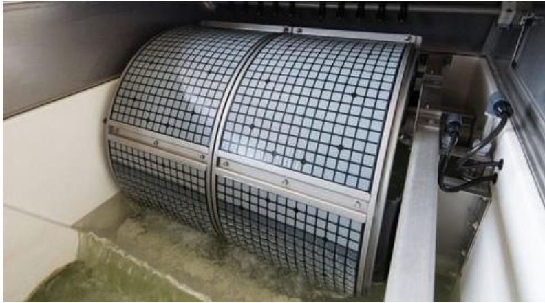
Figure 1.4. Picture of a drum filter, a popular solid removal unit for recirculating aquaculture systems. Source: Global RAS Fishery & Co
