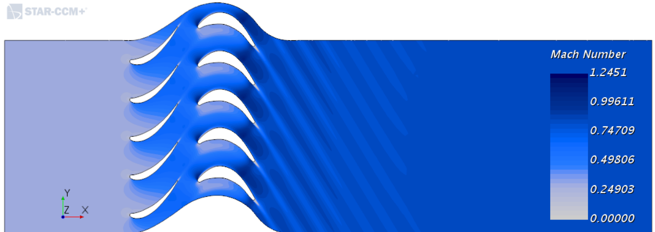
Figure A.23: Zoom of the mach number contour for blade ratio of 1 for Rotor 1. OE
