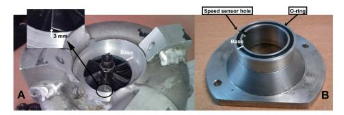
Figure 4: A) Modified compressor housing, B) Coupling piece
