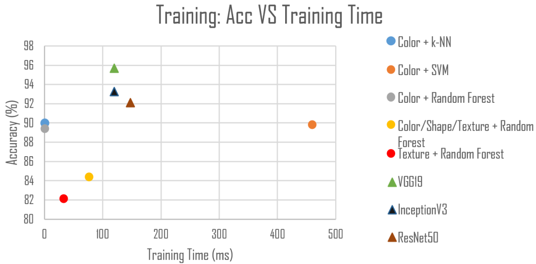
Figure 8.1: Comparison between traditional models and CNNs based on their accuracy and training times (in milliseconds). Circles represent the former, while triangles represent the latter
