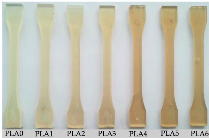
Figure III.3.6. Visual aspect of the injection-molded polylactide (PLA) pieces subjected to different reprocessing cycles.
