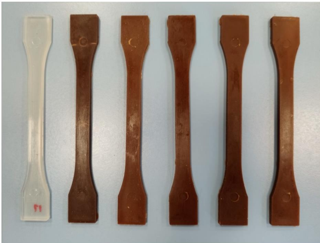
Figure III.4.3. Visual aspect of the polylactide (PLA)/flaxseed flour (FSF) composite pieces processed with epoxidized linseed oil (ELO) and maleinized linseed oil (MLO) corresponding, from left to right, to: PLA, PLA/FSF, PLA/FSF + 2.5ELO, PLA/FSF + 5ELO, PLA/FSF + 2.5MLO, and PLA/FSF + 5MLO.
