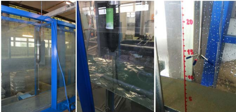
Figure 18. ADV Vectrino by Nortek®, with detail of the receivers, in the classical hydraulic jump experimental device in the Hydraulics Laboratory of the Department of Hydraulic Engineering and Environment at the Universitat Politècnica de València (UPV, Spain).
