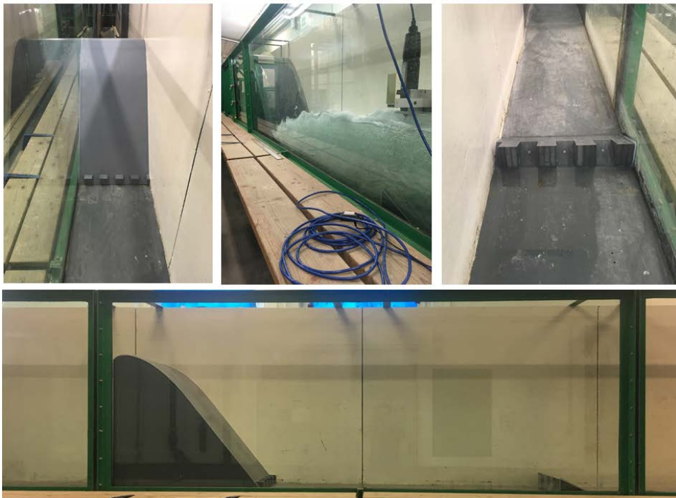
Figure 12. Open flow channel with the typified USBR II stilling basin reduced scale physical model in the Hydraulics Laboratory of the Institute of Hydraulic Engineering and Water Resources Management, at the Technische Universität Wien (TUWien, Austria).
