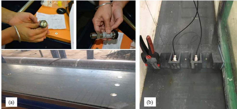
Figure 20. (a) Pressure transmitters and holes to place them in the streambed channel for the classical hydraulic jump in the Hydraulics Laboratory of the Department of Hydraulic Engineering and Environment at the Universitat Politècnica de València (UPV, Spain), (b) Pressure transmitters in the end sill of the typified USBR II stilling basin model in the Hydraulics Laboratory of the Institute of Hydraulic Engineering and Water Resources Management, at the Technische Universität Wien (TUWien, Austria).
