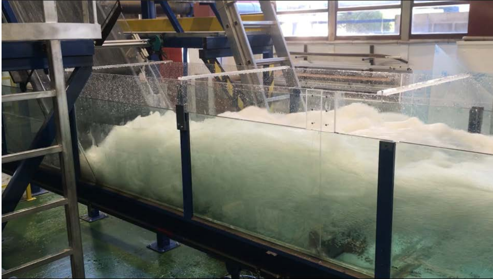
Figure 5. Physical model of a typified USBR II stilling basin in the Hydraulics Laboratory of the Department of Hydraulic Engineering and Environment at the Universitat Politècnica de València (UPV, Spain).
