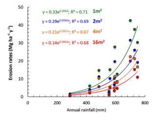
Fig. 6. Relationship between erosion rates and annual rainfall in each plot size.
