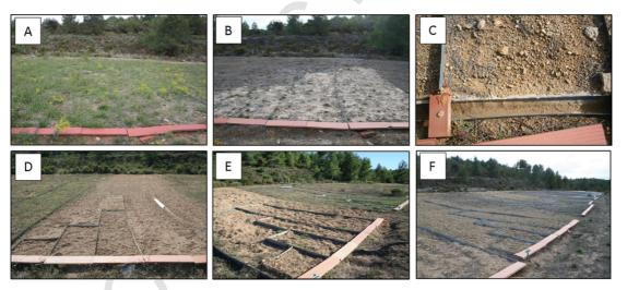
Fig. 2. View of the plots. A: Straw covered plot in spring; B: Straw covered plots in winter; C: view of the runoff collector; D: Control plot in summer after the ploughing; E: Control plot at the end of summer; F: View of the Control plot in winter.
