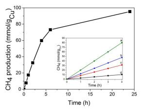
**Fig. 4** CH<sub>4</sub> temporal profile (mmol/g<sub>cu</sub>) at 250 °C for 24 h. Inset shows CH<sub>4</sub> time-production (mmol/g<sub>cu</sub>) at different temperatures under illumination with a Xenon lamp of 300 W at different temperatures (a: 250 °C, b: 225 °C, c: 200 °C and d: 150 °C). Reaction conditions: Cu content 0.56 mg. P<sub>H2</sub> = 1.05 bar, P<sub>CO2</sub> = 0.25 bar.
