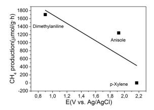
**Fig. 5.** CH<sub>4</sub> production as function of the sacrificial agent oxidation potential. The CH<sub>4</sub> production rate was measured under constant light intensity of 200 mW/cm<sup>2</sup> from a 300 W Xe lamp at 200 °C. Reaction time was 1h. P<sub>H2</sub> =1.05 bar, P<sub>CO2</sub>=0.25 bar. 20  $\mu$ l of each sacrificial agent was added to the reactor vessel in each experiment.
