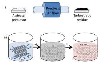
Scheme 1. Cu<sub>2</sub>O/G photocatalyst preparation. i) Pyrolysis of the alginate precursor and ii) dispersion of the turbostratic residue in ethylene glycol (EG) upon 700 W sonication for 1 h (a) and subsequent Cu(NO<sub>3</sub>)<sub>2</sub> addition (b) and reduction at 120 °C for 24 h.
