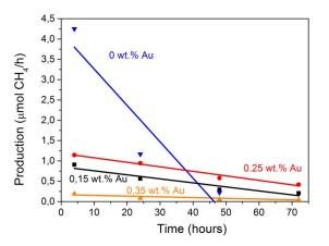
Fig. 8 CH<sub>4</sub> production rate using 0, 0.15, 0.25 and 0.35 wt.%. Au loading in the Cu<sub>2</sub>O/G photocatalyst. The CH<sub>4</sub> production rate
