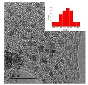
Fig. 2 HRTEM image of  $Cu_2O/G$ , in the centre of the image the size of a representative  $Cu_2O$  NP is indicated. The inset shows size distribution histogram. Scale bar is 20 nm.
