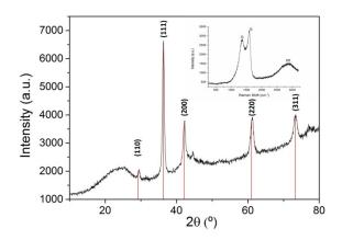
Fig. 1 XRD pattern of the  $Cu_2O/G$  photocatalyst. The peaks corresponding to  $Cu_2O$  have been indicated in red. Inset shows the Raman spectrum of  $Cu_2O/G$  recorded upon 512 nm laser excitation.
