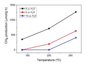
Fig. 6 CH<sub>4</sub> production rate in function of temperature upon addition of H<sub>2</sub>O aliquots. The CH<sub>4</sub> production rate was measured under constant light intensity of 200 mW/cm<sup>2</sup> from a 300 W Xenon lamp. Reaction time was 1h.  $P_{H2}$  =1.05 bar,  $P_{CO2}$ =0.25 bar.
