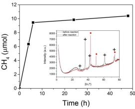
**Fig. 7** Time-CH<sub>4</sub> evolution plot in a 48 h photoassisted methanation using Cu<sub>2</sub>O/G photocatalyst. The inset shows the XRD pattern of just prepared Cu<sub>2</sub>O/G photocatalyst (black crosses) and after submitting it 4 h under the photoassisted reaction conditions (red dots). Reaction conditions: Cu content 0.56 mg. P<sub>H2</sub> = 1.05 bar, P<sub>CO2</sub> = 0.25 bar, temperature 250 °C, irradiation power density 200 mW/cm<sup>2</sup> from a 300 W Xe lamp.
