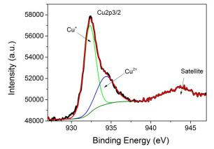
Fig. 3 High resolution XPS peak for Cu2p recorded for  $Cu_2O/G$  sample showing also its best deconvolution to individual components.
