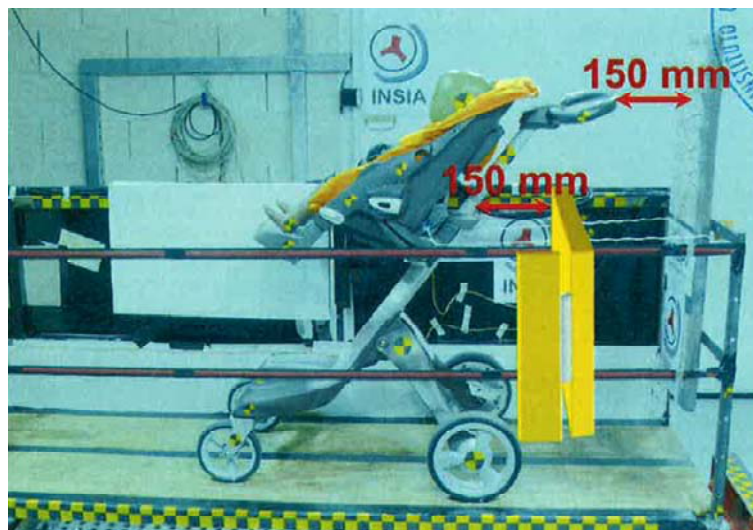
Fig. 7 Superimposed image of test configurations E02 (ASUCAR prototype No. 1) vs. E03 (fixed back-restraint panel for wheelchair passengers) using the SX pushchair.
