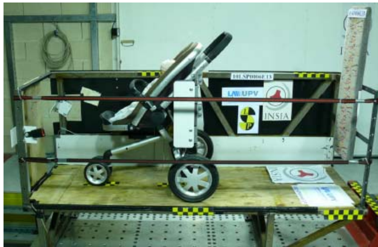
Fig. 3 Rear wall restraint panel for wheelchair passenger and pushchair restraint system mounted on the sled.
