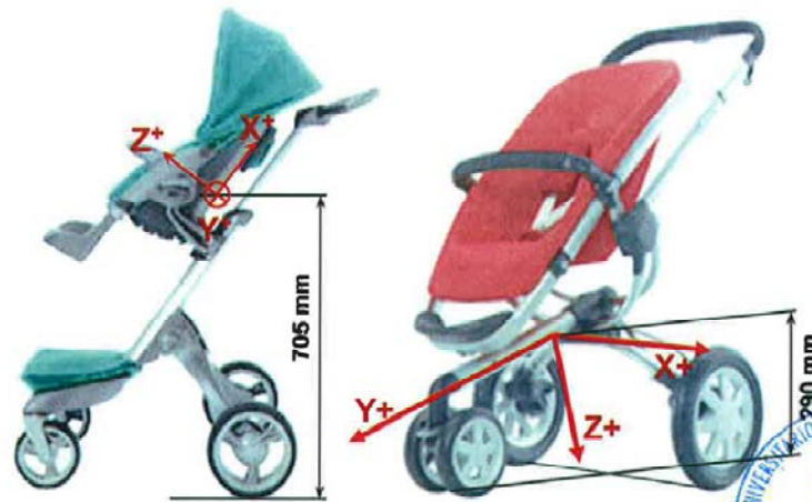
Fig. 4 Position of the accelerometer installed on the pushchairs and reference systems used during dynamic tests (left: SX; right: QB).
