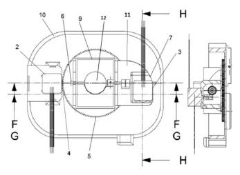
Figure 4. Schematic illustration of the 3D positioning system. The figure on the left shows the top view of the plant and on the right a side view showing the cutting G is depicted. 1-Sample platform, 2-Rotation engine, 3-Angular engine, 4-Rotation power gear, 5-Rotation gear, 6-Shaft, 7-Gearbox, 9-Inner container, 10-Ice container, 11-Structural support, 12-Samples platform.[16]
