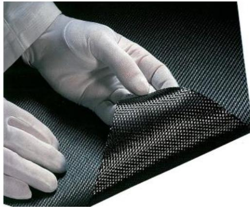
Figura 2.6: Prepeg Carbono-Epoxi [6].
